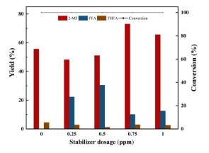
Fig. 4 Effect of stabilizer dosage on furfural selective hydrodeoxygenation conversion and yield using Co/CoO<sub>x</sub>-300 catalysts. Reaction conditions: furfural 2 g, isopropyl 40 mL, catalyst 200 mg, temperature 170 °C, agitation speed 700 rpm, H<sub>2</sub> pressure 2 MPa, time 2 h. 2-MF: 2-methylfuran, FFA: furfuryl alcohol, THFA: tetrahydrofurfuryl alcohol.
