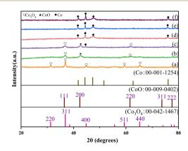
Fig. 1 XRD patterns of (a) unreduced Co/CoO $_{\rm x}$ , (b) 200 °C reduced Co/CoO $_{\rm x}$ , (c) 250 °C reduced Co/CoO $_{\rm x}$ , (d) 300 °C reduced Co/CoO $_{\rm x}$  and (e) 350 °C reduced Co/CoO $_{\rm x}$ .
