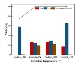
Fig. 2 Effect of reduction temperature on furfural selective hydrodeoxygenation conversion and yield using  $\text{Co/CoO}_x$  catalysts. Reaction conditions: furfural 2 g, isopropyl 40 mL, catalyst 200 mg, agitation speed 700 rpm,  $\text{H}_2$  pressure 2 MPa, temperature 130 °C, time 2 h. 2-MF: 2-methylfuran, FFA: furfuryl alcohol, THFA: tetrahydrofurfuryl alcohol.
