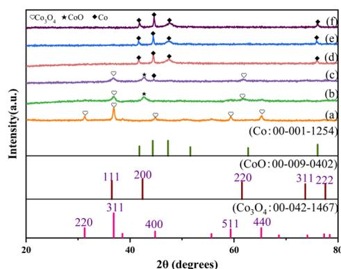
Fig. 1 XRD patterns of (a) unreduced Co/CoO<sub>x</sub>, (b) 200 °C reduced Co/CoO<sub>x</sub>, (c) 250 °C reduced Co/CoO<sub>x</sub>, (d) 300 °C reduced Co/CoO<sub>x</sub> and (e) 350 °C reduced Co/CoO<sub>x</sub>.
