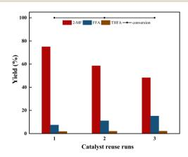
Fig. 5 Reusability of the catalyst for furfural selective hydrodeoxygenation conversion and yield using  $Co/CoO_x$ -300 catalysts. Reaction conditions: furfural 2 g, isopropyl 40 mL, catalyst 200 mg, stabilizer dosage 0.75 ppm, temperature 170 °C, agitation speed 700 rpm,  $H_2$  pressure 2 MPa, time 2 h. 2-MF: 2-methylfuran, FFA: furfuryl alcohol, THFA: tetrahydrofurfuryl alcohol.
