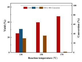
Fig. 3 Effect of reaction temperature on furfural selective hydrodeoxygenation conversion and yield using Co/CoO<sub>x</sub>-300 catalysts. Reaction conditions: furfural 2 g, isopropyl 40 mL, catalyst 200 mg, agitation speed 700 rpm, H2 pressure 2 MPa, time 2 h. 2-MF: 2methylfuran, FFA: furfuryl alcohol, THFA: tetrahydrofurfuryl alcohol.
