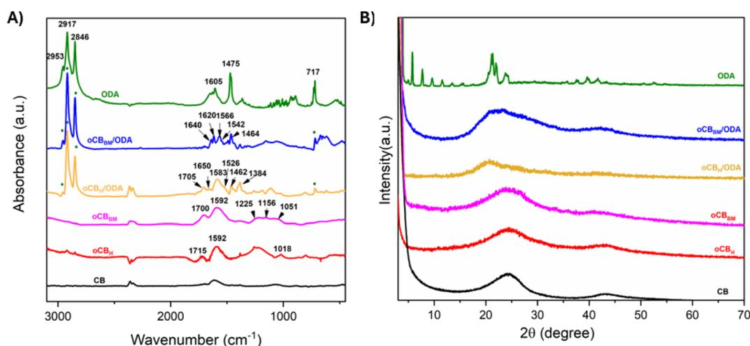
Fig. 1 FTIR (A) and X-ray diffraction patterns (B) of CB (black), oCB<sub>H</sub> (red), oCB<sub>BM</sub> (pink), oCB<sub>H</sub>/ODA (yellow), oCB<sub>BM</sub>/ODA (blue), and ODA (green).
