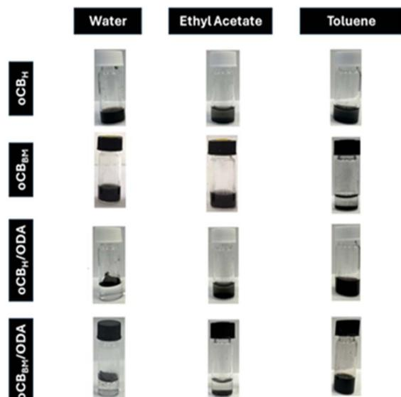
Fig. 3  $\text{oCB}_H$ ,  $\text{oCB}_{BM}$ ,  $\text{oCB}_H/\text{ODA}$ , and  $\text{oCB}_{BM}/\text{ODA}$  suspension in water, ethyl acetate, and toluene solution  $5 \text{ mg mL}^{-1}$  after 5 min of sonication and 30 min of storage.
