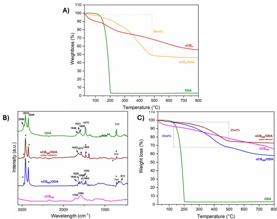
Fig. 2 (A) TGA of oCB<sub>H</sub> (red), ODA (green), and oCB<sub>H</sub>/ODA (yellow); (B) FTIR and (C) TGA of oCB<sub>BM</sub>/ODA before (blue) and after washing (pink) in comparison with oCB<sub>BM</sub> (pink) and ODA (green).
