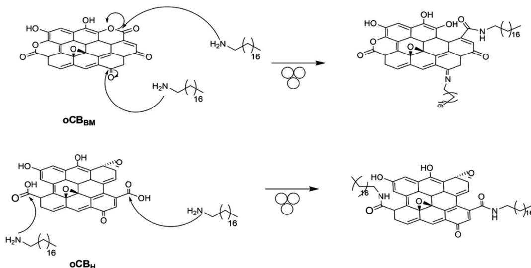
Scheme 1 Mechanism of functionalization of oCB<sub>BM</sub> and oCB<sub>H</sub> with ODA.
