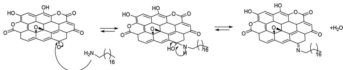
Scheme 2 Mechanism of imine formation of  $\text{oCB}_{\text{BM}}$  with ODA.
