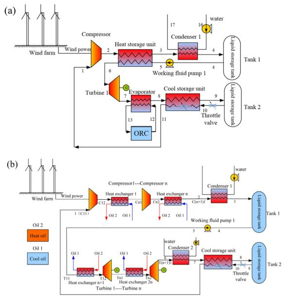
Fig. 5 Various compressed CO<sub>2</sub> energy storage systems: (a) a carbon dioxide energy storage system with a phase transition device; 61 (b) an energy storage system with a combination of wind energy and carbon dioxide.<sup>61</sup>
