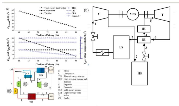
Fig. 4 (a) Compressed  $CO_2$  energy storage system based on Brayton cycle;<sup>59</sup> (b) integrated energy storage system of supercritical (transcritical)  $CO_2$  Rankine cycle and voltage shrinking refrigeration cycle;<sup>60</sup> (c) effect of turbine efficiency on exergy.<sup>59</sup>
