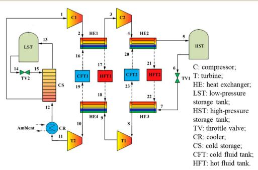
Fig. 6 A new triple production system based on transcritical Brayton cycle and carbon dioxide energy storage.<sup>62</sup>
