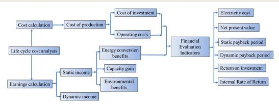
Fig. 9 Flowchart of calculation of life cycle cost analysis.
