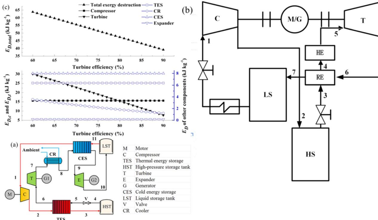
Fig. 4 (a) Compressed CO<sub>2</sub> energy storage system based on Brayton cycle;<sup>59</sup> (b) integrated energy storage system of supercritical (transcritical) CO<sub>2</sub> Rankine cycle and voltage shrinking refrigeration cycle;<sup>60</sup> (c) effect of turbine efficiency on exergy.<sup>59</sup>
