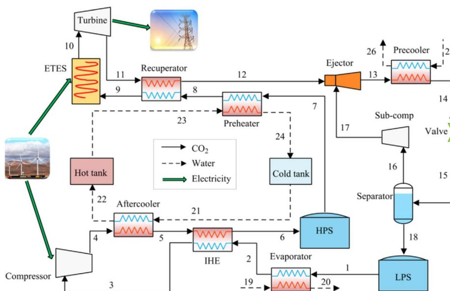
Fig. 2 A schematic of the carbon dioxide electrothermal energy storage system's cycle.<sup>43</sup>
