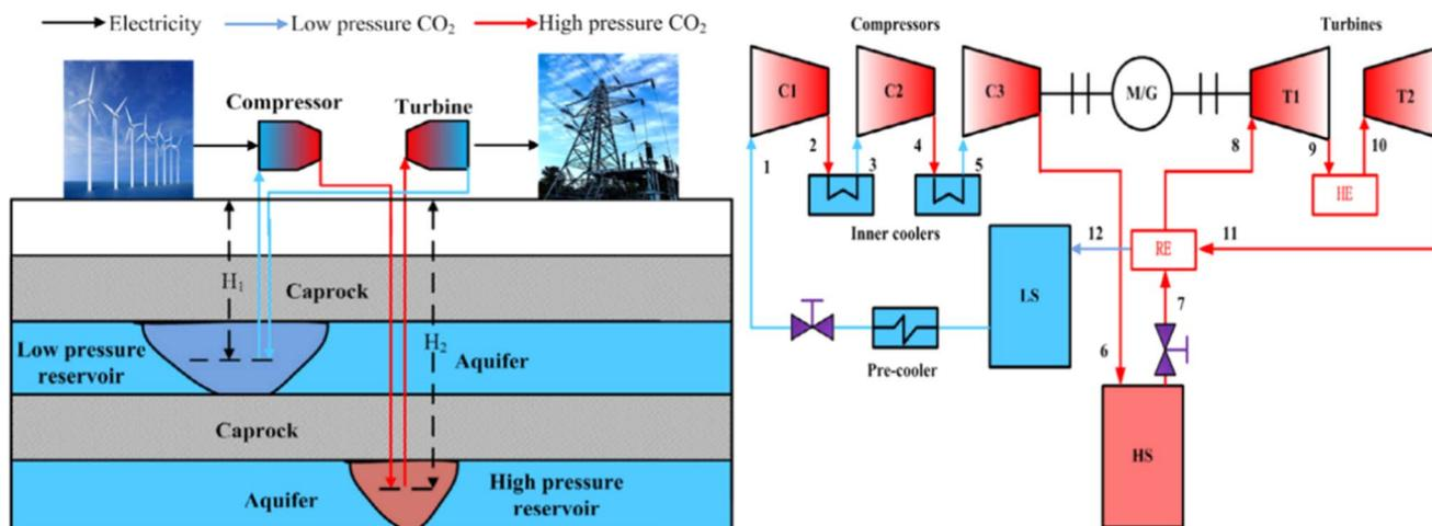
Fig. 7 A carbon dioxide energy storage system with underground rock strata.<sup>47</sup>
