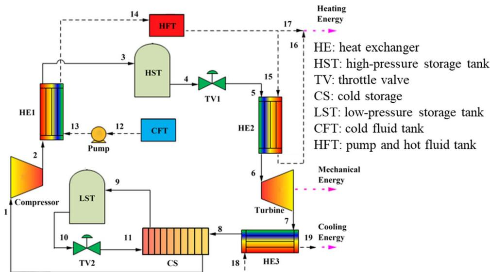
Fig. 3 Schematic diagram of CCES system.<sup>46</sup>
