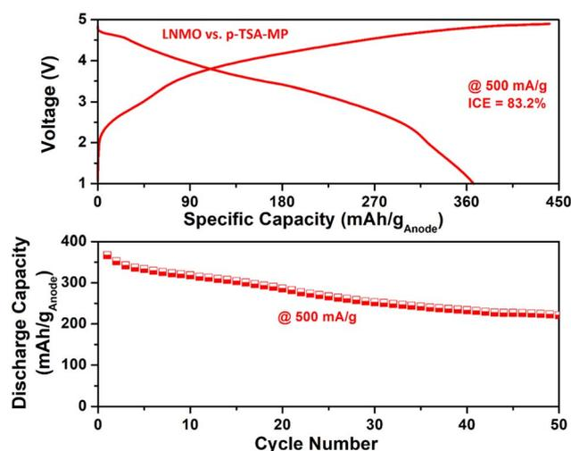
Fig. 6 Electrochemical analysis of LNMO vs. *p*-TSA-MP: (a) voltage vs. specific capacity ( $\text{mA h g}_{\text{anode}}^{-1}$ ) and (b) discharge capacity ( $\text{mA h g}_{\text{anode}}^{-1}$ ) vs. cycle number of LNMO vs. *p*-TSA-MP at a current of  $500 \text{ mA g}^{-1}$  for 50 cycles.
