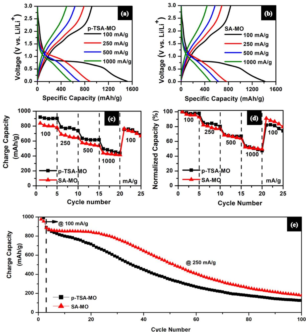
Fig. 7 (a) and (b) The first charge–discharge profile in a voltage window 0.01–3.0 V, (c) and (d) rate performance and normalized capacity (%), and (e) cycling performance cycled at 100 and 250 mA g<sup>-1</sup> for mixed metal oxides *p*-TSA-MO and SA-MO.
