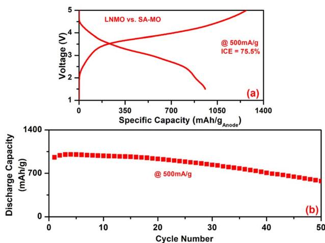
Fig. 8 Electrochemical analysis of LNMO vs. SA-MO: (a) voltage vs. specific capacity (mA h g<sub>anode</sub><sup>-1</sup>) and (b) discharge capacity (mA h g<sub>anode</sub><sup>-1</sup>) vs. cycle number at a current of 500 mA g<sup>-1</sup> for 50 cycles.
