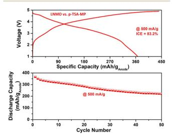
Fig. 6 Electrochemical analysis of LNMO vs. p-TSA-MP: (a) voltage vs. specific capacity (mA h  $g_{anode}^{-1}$ ) and (b) discharge capacity (mA h  $g_{anode}^{-1}$ ) vs. cycle number of LNMO vs. p-TSA-MP at a current of 500 mA  $g^{-1}$  for 50 cycles.
