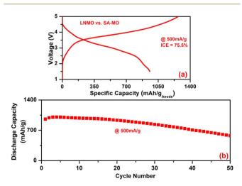
Fig. 8 Electrochemical analysis of LNMO vs. SA-MO: (a) voltage vs. specific capacity (mA h  $g_{anode}^{-1}$ ) and (b) discharge capacity (mA h  $g_{anode}^{-1}$ ) vs. cycle number at a current of 500 mA  $g^{-1}$  for 50 cycles.
