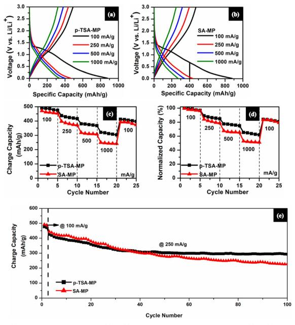
Fig. 5 (a) and (b) The first charge—discharge profile, (c) and (d) the rate performance and normalized capacity (%) and (e) cycling at 100 and 250 mA  $g^{-1}$  of mixed metal phosphides for p-TSA-MP and SA-MP.
