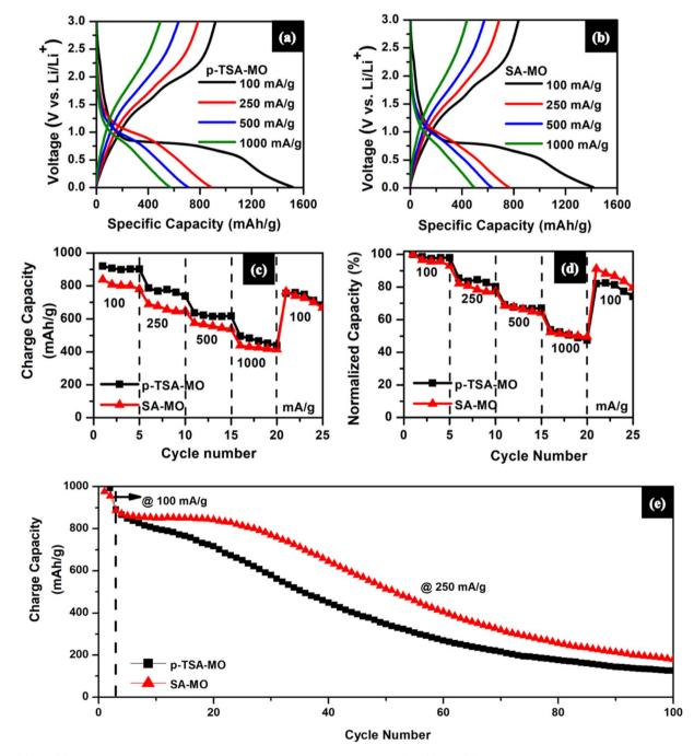
Fig. 7 (a) and (b) The first charge–discharge profile in a voltage window 0.01–3.0 V, (c) and (d) rate performance and normalized capacity (%), and (e) cycling performance cycled at 100 and 250 mA  $\rm g^{-1}$  for mixed metal oxides p-TSA-MO and SA-MO.
