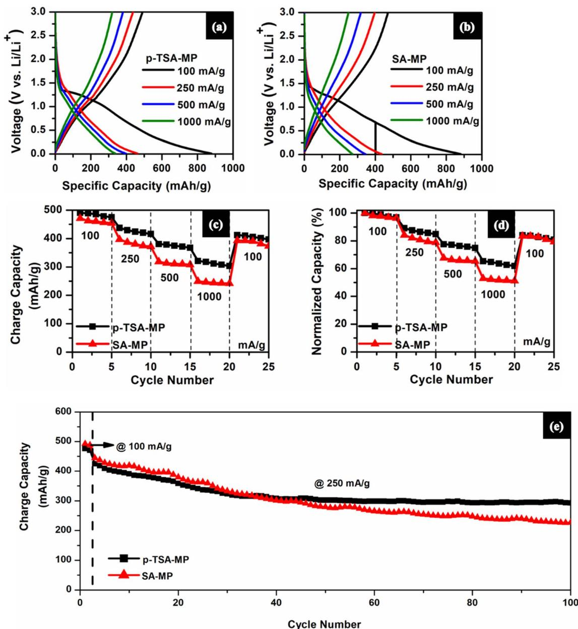
Fig. 5 (a) and (b) The first charge–discharge profile, (c) and (d) the rate performance and normalized capacity (%) and (e) cycling at 100 and 250 mA g<sup>-1</sup> of mixed metal phosphides for *p*-TSA-MP and SA-MP.
