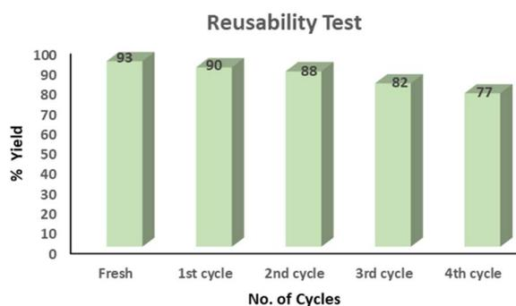
Fig. 1 Reusability test of the DES. Reaction conditions: *p*-tolualdehyde (1.56 mmol), diethylamine (1.56 mmol) and sulfur powder (0.195 mmol) in 25 mol% DES ChCl-urea (1 : 2) at 45 °C for 5 h. Isolated yields.
