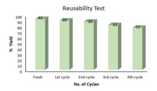
Fig. 1 Recyclability test of the DES. Reaction conditions: p-tolualdehyde (1.56 mmol), diethylamine (1.56 mmol) and sulfur powder (0.195 mmol) in 25 mol% DES ChCl-urea (1:2) at 45 °C for 5 h. Isolated yields.
