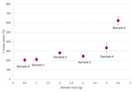
Fig. 3 Temperatures reached by the spent LCO battery samples, treated at 600 W for 5 minutes, as a function of the samples' mass. Error bars correspond to the temperature variation inside the samples, evaluated by the thermal imaging camera.
