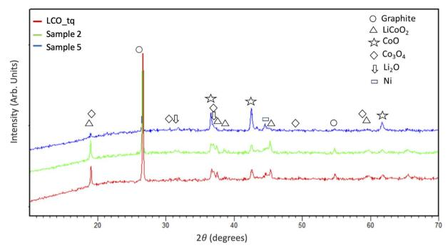
XRD patterns of LCO BM before (sample LCO\_tq) and after MW treatment with the increase of black mass (sample 2 and sample 5).
