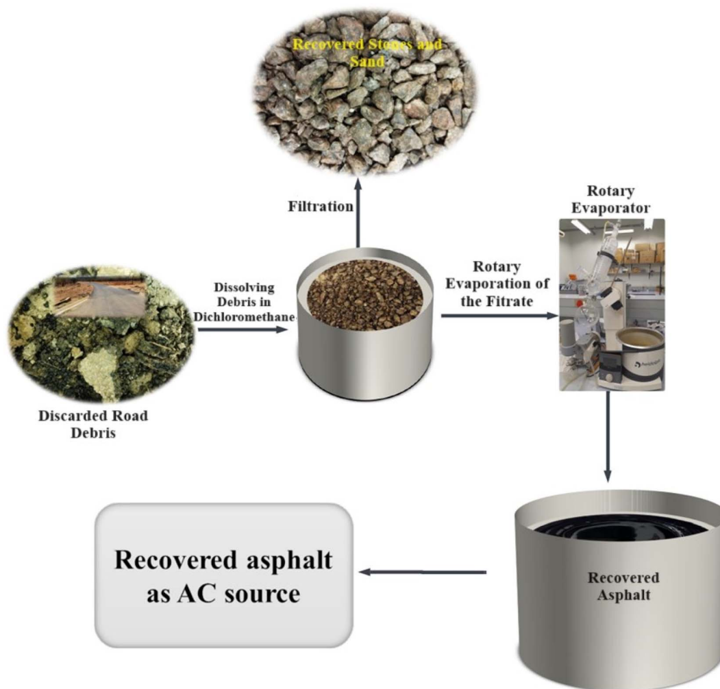
Fig. 1 A schematic illustration of asphalt recovery process.
