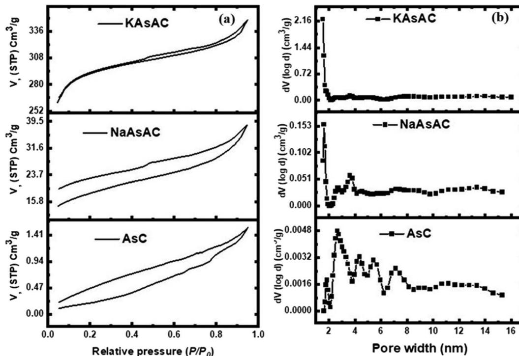
Fig. 7  $N_2$  adsorption–desorption isotherms and pore width distribution of AsC, NaAsAC, and KAsAC samples.
