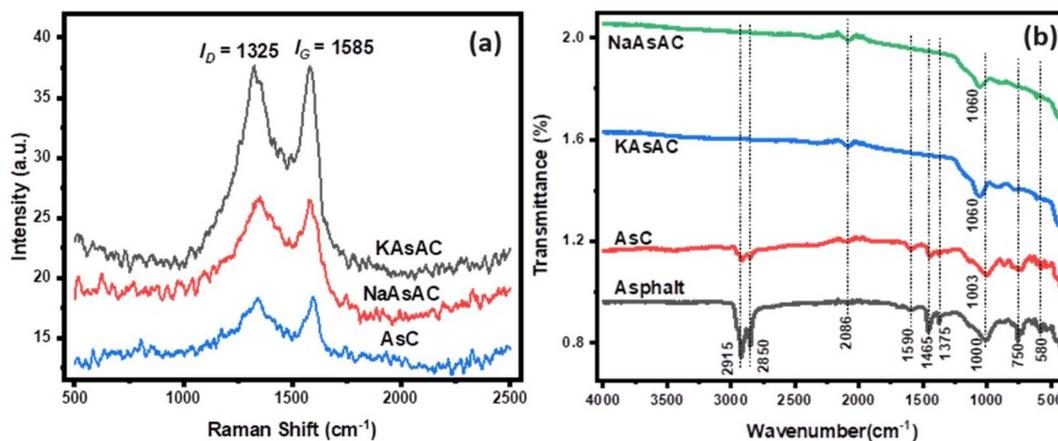
Fig. 4 (a) Raman spectra of the prepared samples from asphalt and (b) FTIR spectra for asphalt and the prepared samples.
