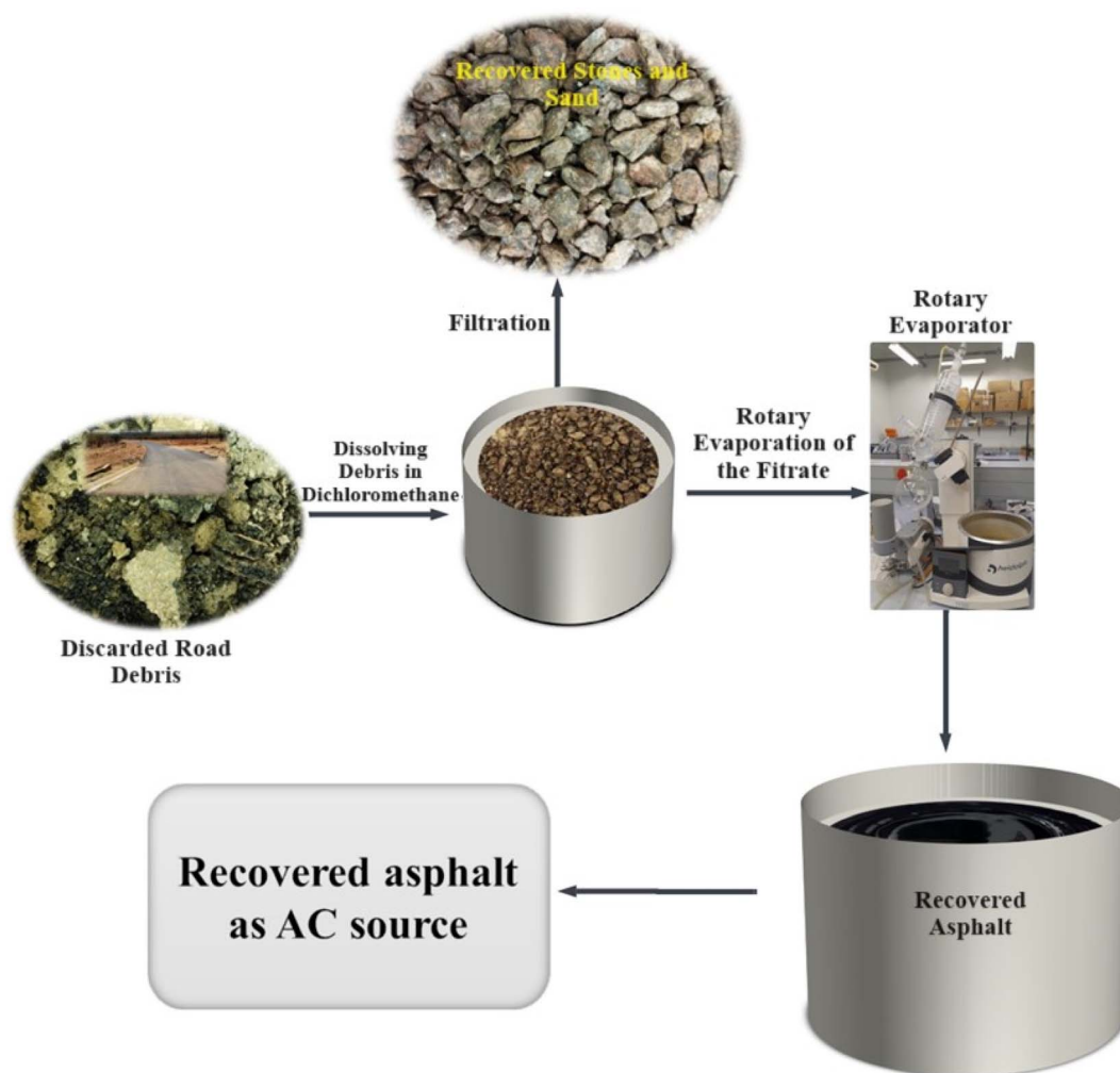
Fig. 1 A schematic illustration of asphalt recovery process.
