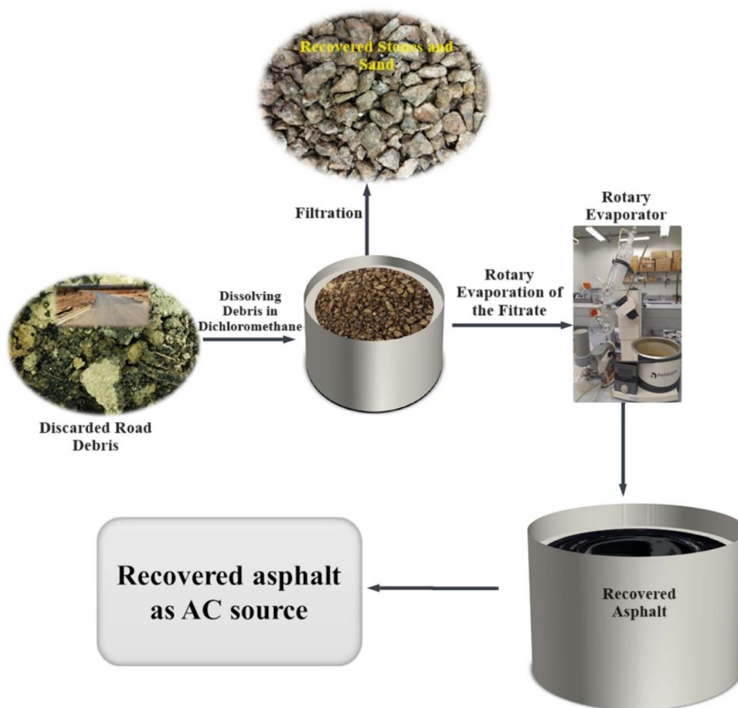
Fig. 1 A schematic illustration of asphalt recovery process.
