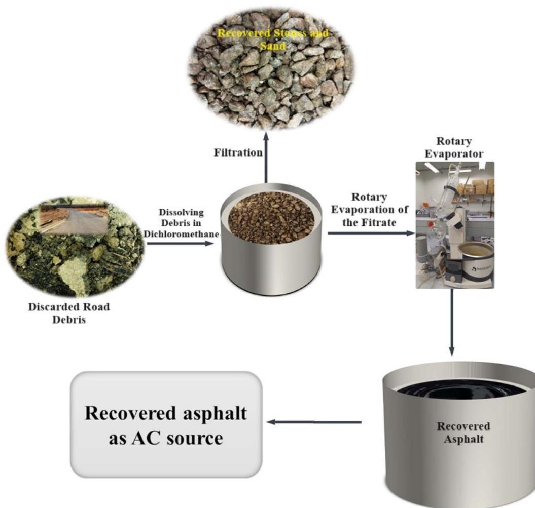
Fig. 1 A schematic illustration of asphalt recovery process.
