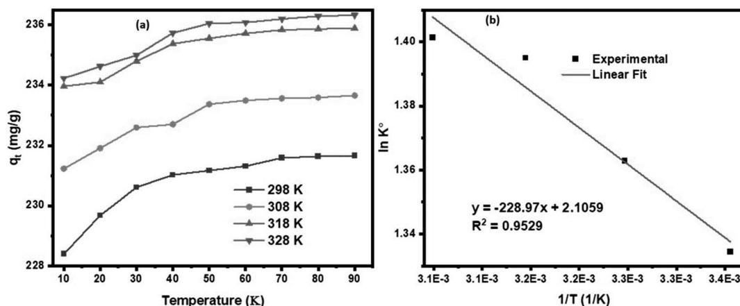
Fig. 11 (a) Effects of temperature on the DP over KAsAC, (b) van't Hoff plot for DP sorption onto KAsAC.
