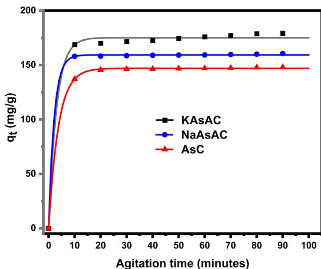
Fig. 8 Effect of adsorption time on DP over AsC, NaAsAC, and KAsAC sorbents.
