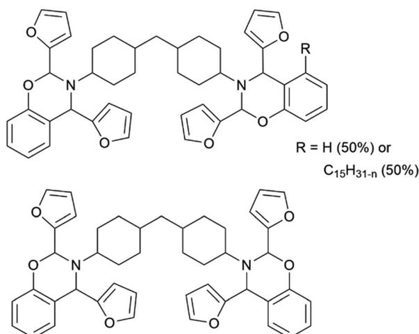
Fig. 1 Idealised structures of FUROX BDP4740 (above) and FUROX FB601 structure (below).
