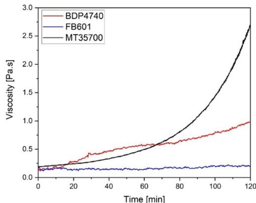
Fig. 5 Time-dependent viscosity curves of BDP4740 and FB601 at 100 °C as well as of MT3700 at 140 °C.
