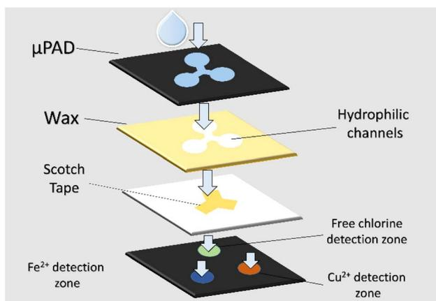
Fig. 4 Design of simultaneous monitoring  $\mu$ PAD for free chlorine,  $\text{Cu}^{2+}$  and  $\text{Fe}^{2+}$ .<sup>62</sup>
