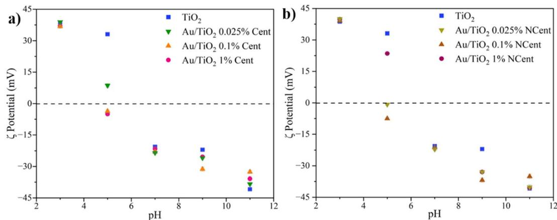
Fig. 6 Zeta potential of pristine  $\text{TiO}_2$  and  $\text{Au/TiO}_2$  nanoparticles, both (a) centrifuged and (b) non-centrifuged.
