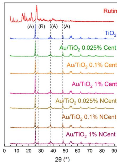
Fig. 4 XRD reflexes of rutin, pristine  $\text{TiO}_2$  and synthesised  $\text{Au/TiO}_2$  nanoparticles, both centrifuged (Cent) and non-centrifuged (NCent), showing the peaks corresponding to the anatase (A) and rutile (R) crystalline phases.
