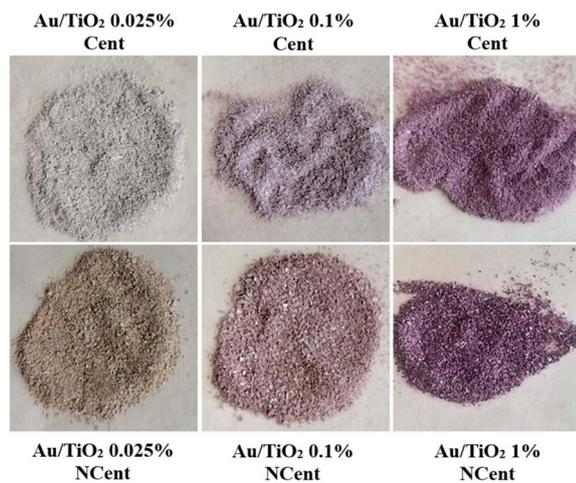
Fig. 2 Influence of different Au concentrations and presence of rutin on the synthesised nanoparticles' colour.
