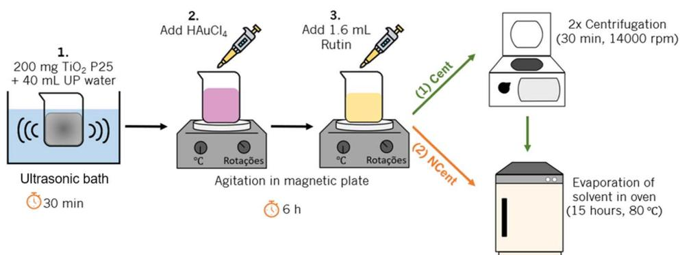
Fig. 1 Schematic representation of the Au/ $TiO_2$  synthesis process.
