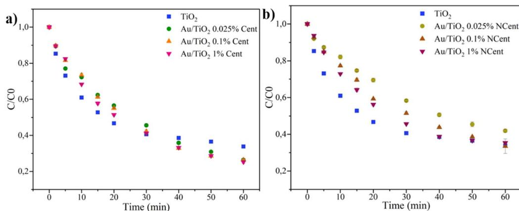
**Fig. 9** Photocatalytic degradation of CIP ( $5 \text{ mg L}^{-1}$ ) under UV radiation for 60 minutes for pristine  $\text{TiO}_2$  and synthesized Au/ $\text{TiO}_2$  nanoparticles, both (a) centrifuged and (b) non-centrifuged.
