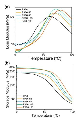
Fig. 5 DMA results showing (a) loss modulus (E'') and the (b) storage modulus (E') curves for neat PA66 and flame-retardant polyamide series.
