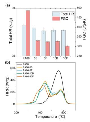
Fig. 4 (a) Total heat release of pure PA66 as compared to both blended and functionalised samples. The presence of DOPO decreased the total HR significantly. The FGC is the fire growth capacity, which gives insight into the ignition and subsequent flame growth. (b) MCC results showing heat release rate (HRR) curves for neat PA66 and flame-retardant polyamide series.
