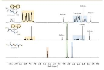
Fig. 1 <sup>1</sup>H NMR spectra of the (a) starting diester (dmt3HD) (b) DOPOgrafted diester in CDCl3 (c) and desired product (DOPO-HDA) in DMSO-d6.
