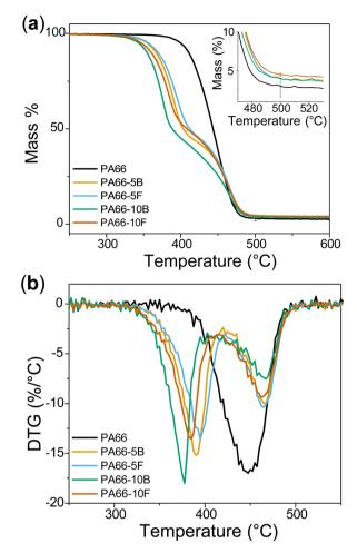
Fig. 3 (a) TGA thermograms for neat PA66 and flame-retardant polyamide series under nitrogen atmosphere. (b) Differential thermogravimetry (DTG) shows the temperature when maximum thermal decomposition occurs.
