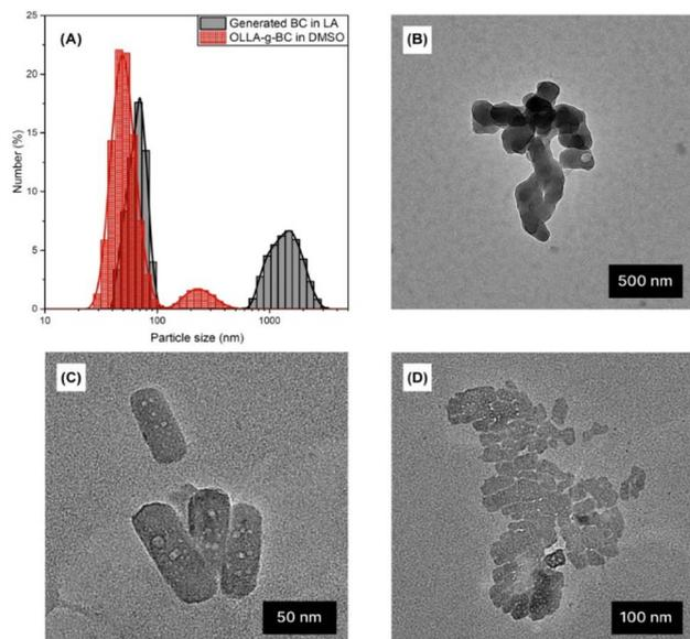
Fig. 3 Size determination of BC and PLLA grafted BC: (A) number-weighted size distributions measured by DLS for OLLA-g-BC in DMSO and regenerated BC in LA. (B) TEM micrographs of aggregates of regenerated BC nanoparticles, (C) quasi-cylindrical OLLA-g-BC nanoparticles, (D) aggregates of OLLA-g-BC nanoparticles.
