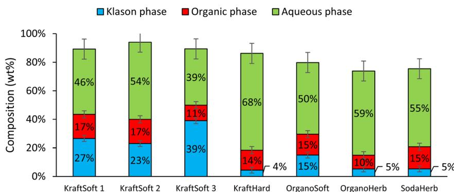
**Fig. 10** Mass balance obtained from the catalytic oxidation of the different lignins, calculated in lignin basis (150 °C, 20 bar of air, 60 minutes, CuO/TiO<sub>2</sub> 5% wt Cu, 5% Cu/lignin).
