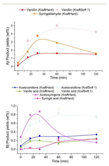
Fig. 13 Product yields obtained by GC analyses of the organic phase, obtained from the catalytic oxidation (5% CuO/TiO<sub>2</sub>, 5% Cu/lignin, 90-200 μm, 150 °C, 20 bar of air and 1800 rpm) of KraftHard (continuous line), and KraftSoft 1 (dotted line).
