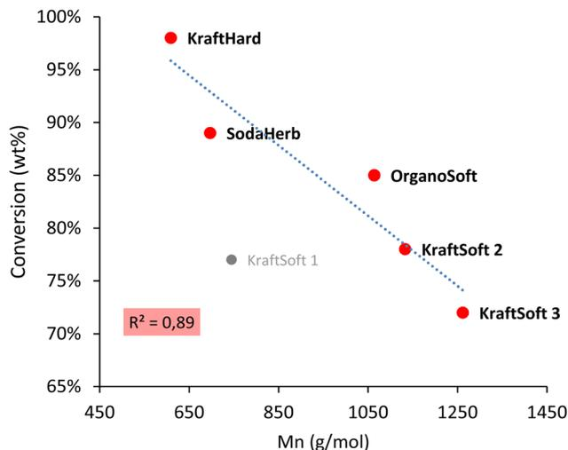
Fig. 6 Correlation between the molecular weight ( $M_n$ ) obtained by the SEC analysis, and conversion obtained by the non-catalytic oxidation reaction.
