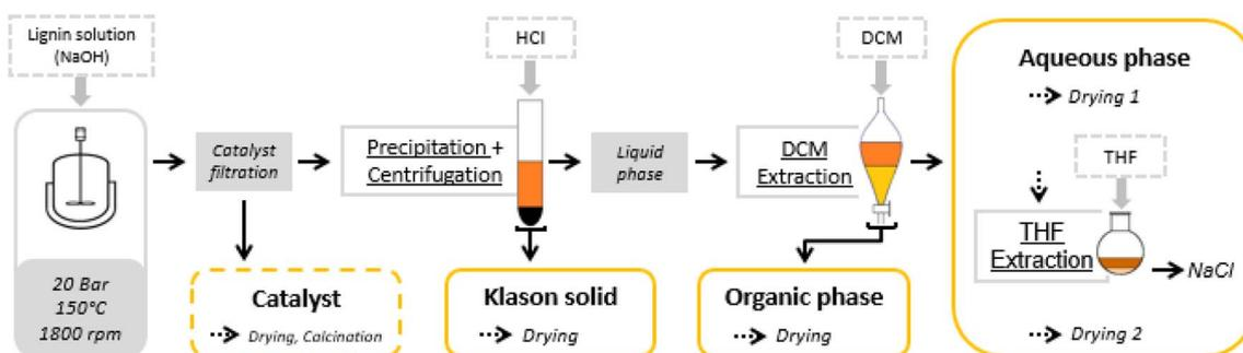
Fig. 1 Oxidation test and fractionation protocol.<sup>55</sup>
