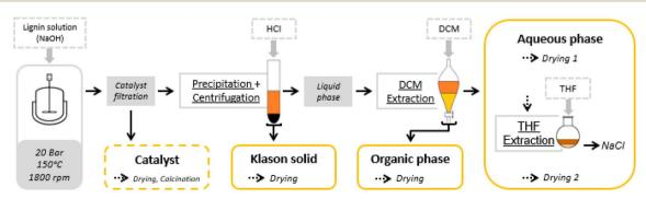
Fig. 1 Oxidation test and fractionation protocol. 55
