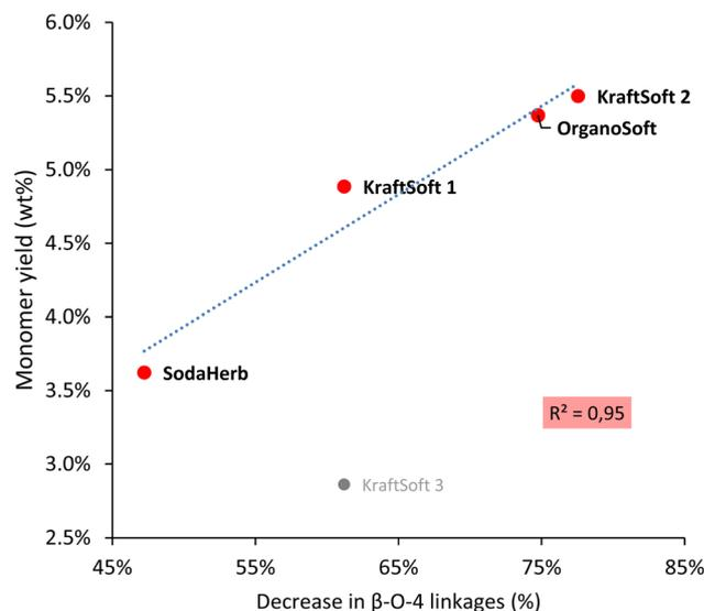
Fig. 9 Correlation between the decrease in the  $\beta$ -O-4 content obtained by HSQC-NMR analysis of the Klason phases, and the monomeric yield obtained from the non-catalytic oxidation reaction of the different lignins under standard conditions.
