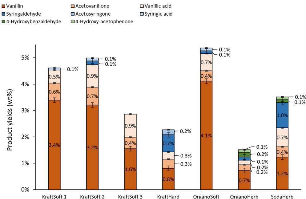
Fig. 7 Yields of aromatics in the organic phases, calculated on lignin basis, obtained from the non-catalytic oxidation of the different lignins (150 °C, 20 bar air, 60 minutes).
