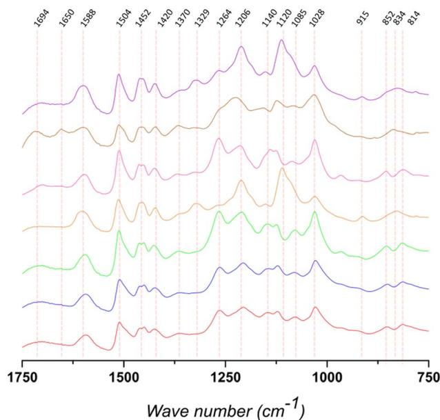
Fig. 2 Extension (1800–750  $\text{cm}^{-1}$ ) of FTIR-ATR spectra of the different lignins: KraftSoft 1 (red), KraftSoft 2 (blue), KraftSoft 3 (green), KraftHard (orange), OrganoSoft (pink), OrganoHerb (brown) and SodaHerb (violet).
