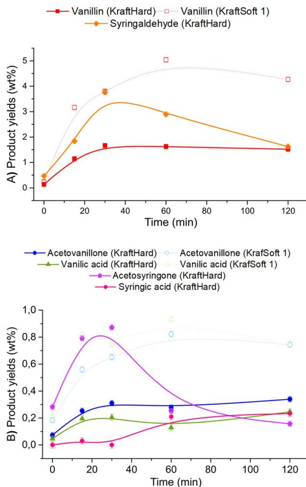
Fig. 13 Product yields obtained by GC analyses of the organic phase, obtained from the catalytic oxidation (5% CuO/TiO<sub>2</sub>, 5% Cu/lignin, 90–200 μm, 150 °C, 20 bar of air and 1800 rpm) of KraftHard (continuous line), and KraftSoft 1 (dotted line).
