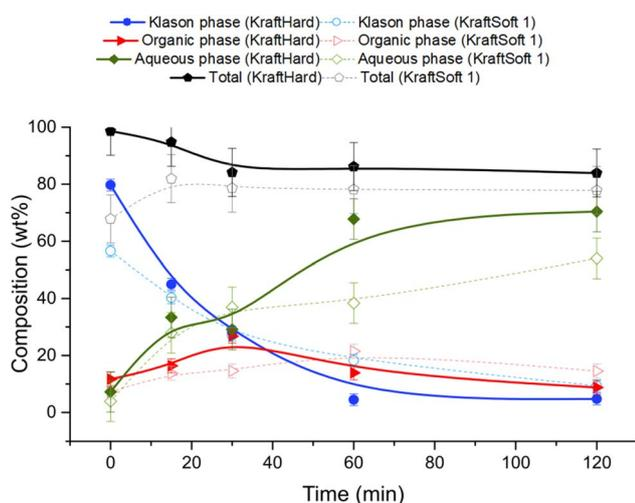
Fig. 12 Mass balance of the different fractions, obtained from the catalytic oxidation (5% CuO/TiO<sub>2</sub>, 5% Cu/lignin, 90–200 μm, 150 °C, 20 bar of air and 1800 rpm) of KraftHard (continuous line), and KraftSoft 1 (dotted line). Each set of points corresponds to one experiment in the bath reactor. Lines are guide for the eyes.
