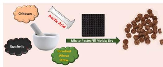
Scheme 1 Schematic representation of blending the powdered constituents into a moulded paste, where the resulting pellets were obtained upon drying. Note that method 1 incorporates ammonium sulfate (AS) during the pellet preparation, whereas method 2 involves incorporation of AS after pellet preparation *via* imbibing pellets in an adsorption process. The black square is the mold for the pellet preparation.
