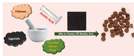
Scheme 1 Schematic representation of blending the powdered constituents into a moulded paste, where the resulting pellets were obtained upon drying. Note that method 1 incorporates ammonium sulfate (AS) during the pellet preparation, whereas method 2 involves incorporation of AS after pellet preparation via imbibing pellets in an adsorption process. The black square is the mold for the pellet preparation.
