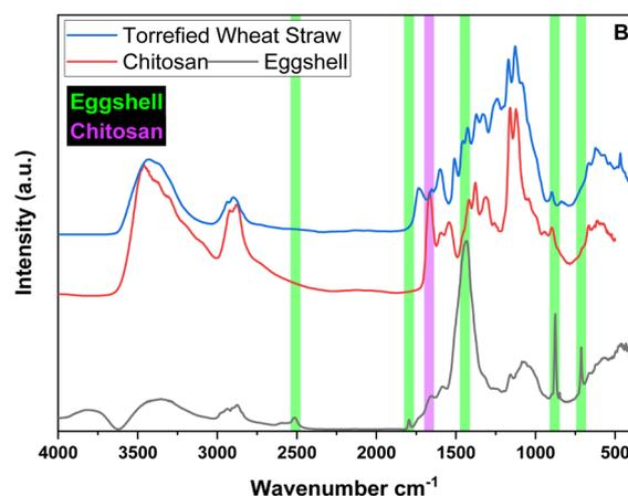
**Fig. 1** FT-IR spectra (normalised) of five types of composites (A) and their respective raw materials (B) with characteristic bands highlighted to support the presence of intact eggshells after composite formation.
