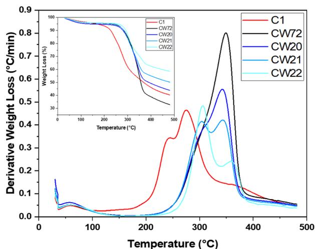
**Fig. 2** DTG profiles of the prepared and for further investigation selected composites (with TG curves as the inset).
