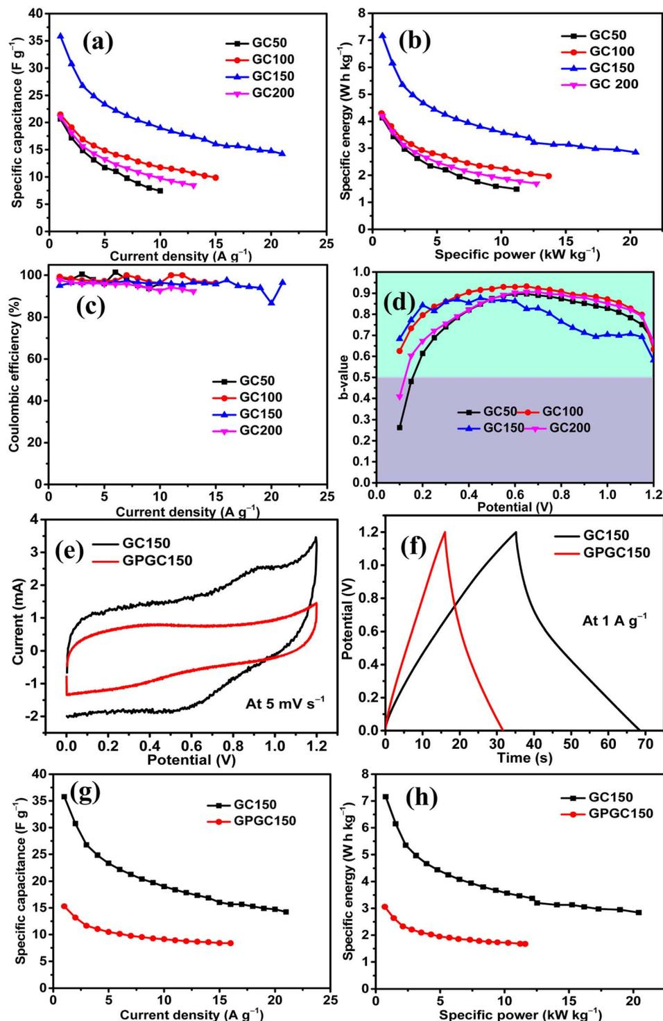
Fig. 6 Plots of (a) specific capacitance vs. current density, (b) specific energy vs. specific power, (c) coulombic efficiency vs. current density, (d)  $b$ -values vs. potential, (e) CV curves at a scan rate of  $5 \text{ mV s}^{-1}$ , (f) CD curves at a current density of  $1 \text{ A g}^{-1}$ , (g) plots of specific capacitance vs. current densities, and (h) plots of specific energy vs. specific power of GC150 and GPGC150.
