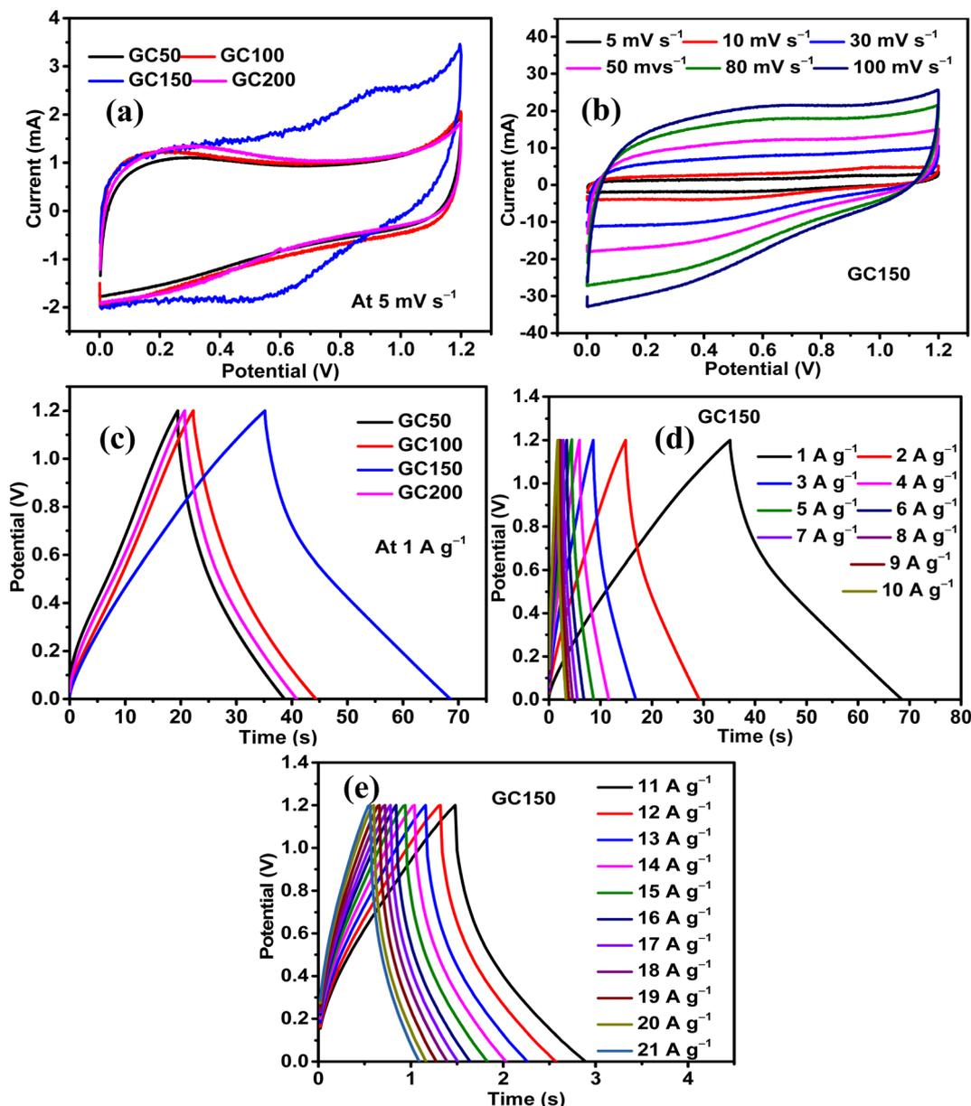
Fig. 5 Cyclic voltammetry (CV) curves of (a) different GC composites at a scan rate of  $5 \text{ mV s}^{-1}$ , (b) GC150 at different scan rates; galvanostatic charge and discharge (GCD) curves of (c) GC composites, (d) GC150 from the current density of 1 to  $10 \text{ A g}^{-1}$ , and (e) GC150 from the current density of 11 to  $21 \text{ A g}^{-1}$ .
