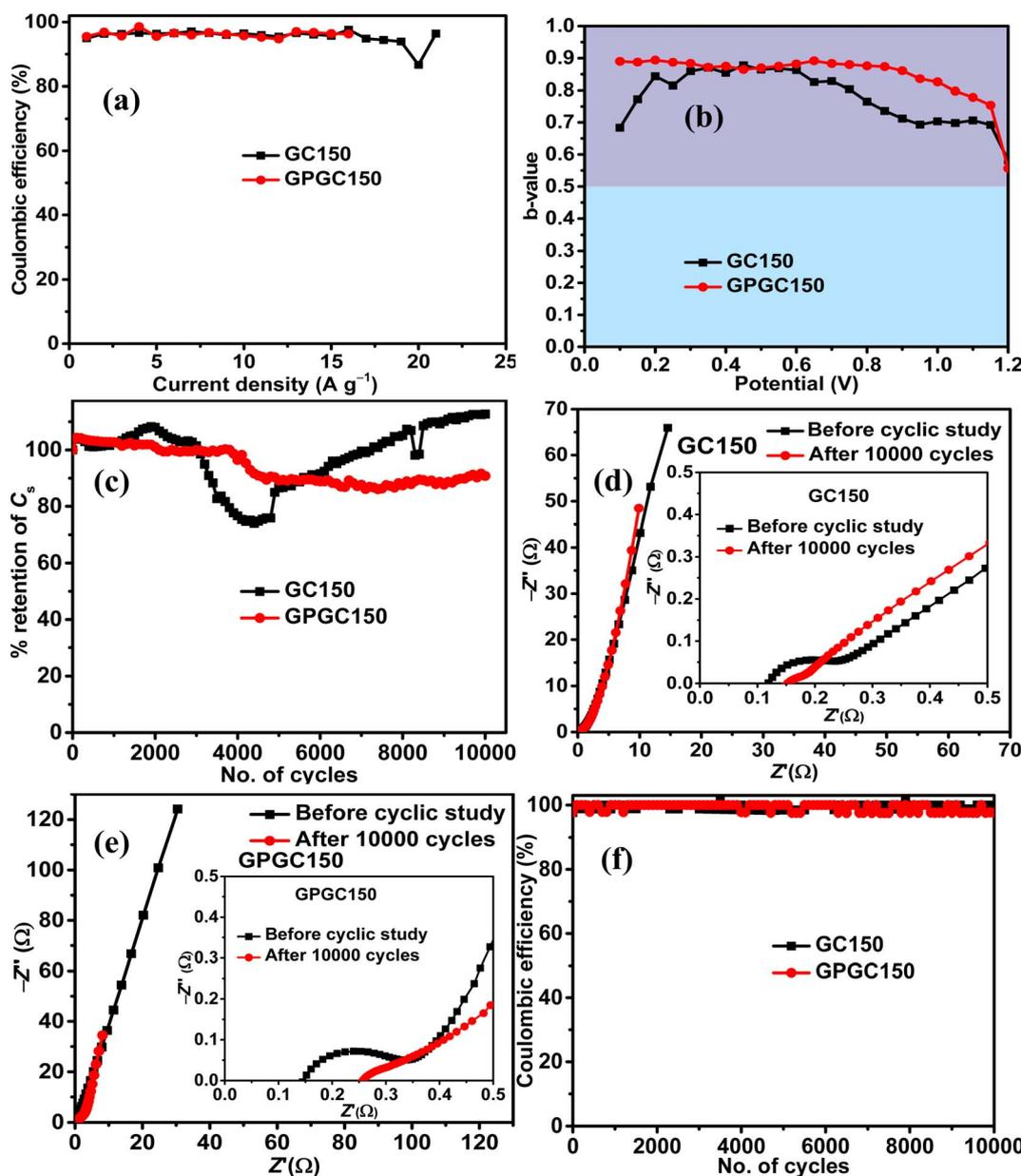
Fig. 7 Plots of (a) coulombic efficiency vs. current density, (b)  $b$ -values vs. potential, (c) %retention of  $C_s$  vs. number of cycles obtained at a current density of  $10 \text{ A g}^{-1}$ , (d) Nyquist plots of GC150 before and after 10 000 cycles, (e) Nyquist plots of GPGC150 before and after 10 000 cycles, and (f) coulombic efficiency vs. no. of cycles obtained at a current density of  $10 \text{ A g}^{-1}$  of GC150 and GPGC150.
