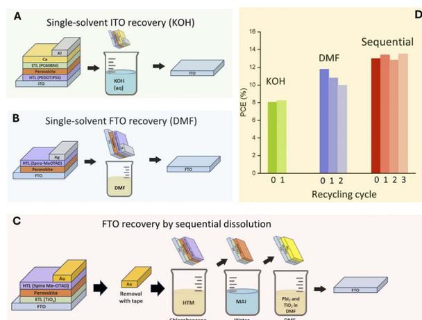
Fig. 1 Schematic of single-solvent TCO-substrate recovery method using (A) an alkaline solution or (B) dimethylformamide. (C) Multi-solvent TCO recovery methods. (D) Performance of the devices fabricated with recycled TCO substrates as reported by Augustine *et al.*,<sup>17</sup> Huang *et al.*<sup>18</sup> and Binek *et al.*<sup>15</sup>
