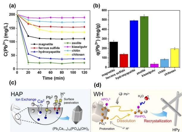
**Fig. 4** (a and b) Performance of different adsorption composites for Pb<sup>2+</sup> retrieval from aqueous solutions (reproduced with permission from ref. 56. Copyright 2021, American Chemical Society). Pb<sup>2+</sup> adsorption mechanisms of (c) hydroxyapatite and (d) whitlockite (reproduced from ref. 55, available under a Creative Commons CC BY licence).
