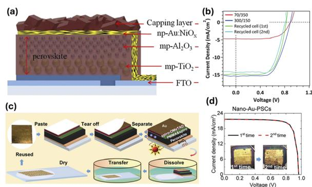
Fig. 5 Alternative designs allowing for gold reuse. (a) Au/NiO<sub>x</sub> is used as HTM/counter electrode in a recyclable all inorganic fully printable stack. (b) JV curves of fresh vs. recycled devices with architecture (Reproduced with permission from ref. 71. Copyright 2017, American Chemical Society). (c) Process for removal and reuse of nano-Au film, (d) performance of devices fabricated with recycled Au film (Reproduced from ref. 72, available under a Creative Commons CC BY licence).
