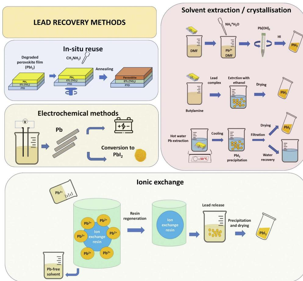
Fig. 3 Schematic of PbI<sub>2</sub> recovery through different methods: *in situ* reuse, electrochemical methods, solvent extraction and crystallisation, and adsorption and ionic exchange.
