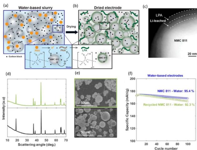
Fig. 7 Schematic representation of the *in situ* formation of lithium polyacrylate during the slurry fabrication (a) and in the final electrode (b). (c) TEM image of the aqueous processed NMC 811 electrode. (d) XRD and (e) SEM images of the pristine (bottom) and recycled (top) NMC 811 cathode material. (f) Galvanostatic cycling of the recycled NMC 811 material in comparison with the pristine one. Reproduced with permission of ref. 153, Copyright 2022, *Journal of Electrochemical Society*.
