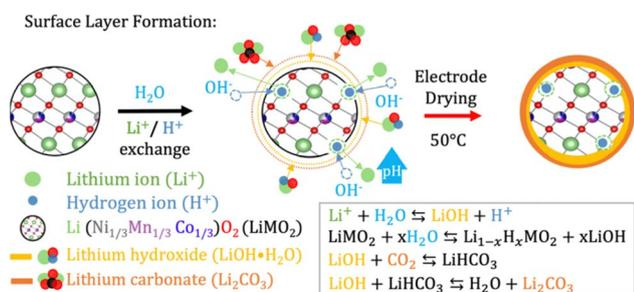
Fig. 3 Scheme of the lithium leaching degradation when nickel-rich NMC are processed *via* aqueous routes. Reproduced with permission of ref. 73, Copyright 2023, Royal Society of Chemistry.
