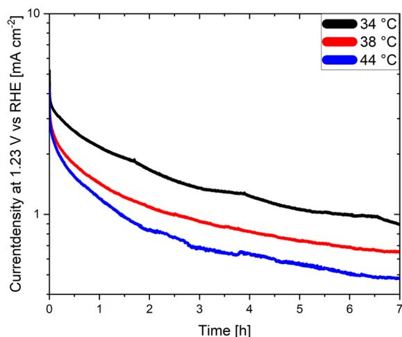
Fig. 6 Chronoamperometries of LaTiO<sub>2</sub>N based photoanodes at 1.23 V vs. RHE in 0.1 M Na<sub>2</sub>SO<sub>4</sub> (pH adjusted to 13.4 with NaOH) at various electrolyte temperatures.
