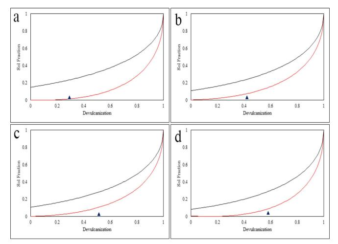
Fig. 14 Horikx plot for (a) S.F<sub>dv</sub>, (b) 40 M<sub>dv</sub>, (c) 80 M<sub>dv</sub>, and (d) 120 M<sub>dv</sub> samples. Below the red curve, selective crosslink scission is happening, the area between the red and black curves shows that crosslink and backbone scission are coinciding, and above the black curve is the region in which the backbone scission is dominant.
