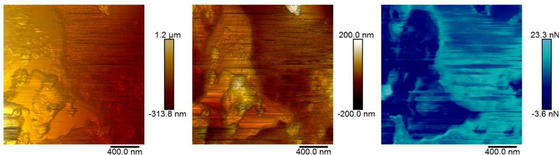
Fig. 8 AFM images of 120  $M_{dv}$  sample, blue the concurrent map of adhesive interaction.
