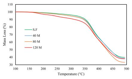
Fig. 16 TGA curves of the devulcanized samples.
