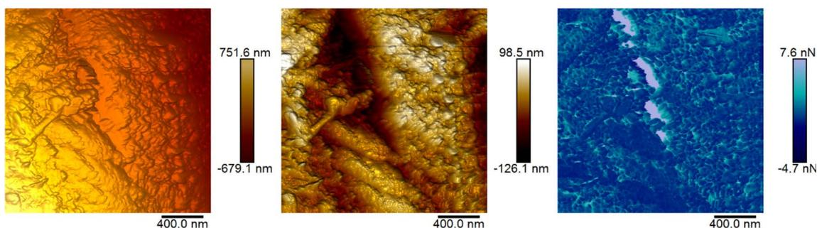
Fig. 7 AFM images of 120  $M_u$  sample, blue the concurrent map of the adhesive interaction.
