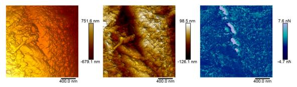
Fig. 7 AFM images of 120 M<sub>II</sub> sample, blue the concurrent map of the adhesive interaction.
