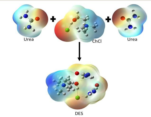
Fig. 1 The chemical structures of ChCl, urea, and ChCl-urea DES (reprinted with permission).<sup>37,38</sup>
