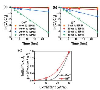
Fig. 5 Kinetic plots of the (a) transport of Co<sup>2+</sup>, (b) transport of Ni<sup>2+</sup>, and (c) initial flux at varying weight composition of the extractant across IEPIM in the feed solution.
