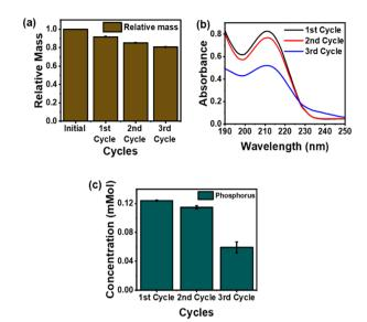
Fig. 4 (a) Mass changes of IEPIM for three cycles (b) UV-Vis spectra showing imidazolium peaks (c) phosphorus concentration in the solution after immersion in deionized water
