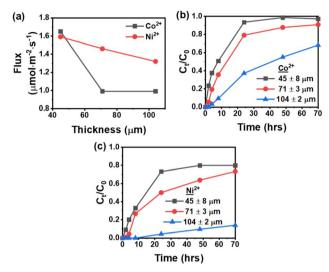
Fig. 7 (a) Initial flux of Co<sup>2+</sup> and Ni<sup>2+</sup> (b) transport efficiency of Co<sup>2+</sup> (c) transport efficiency of Ni<sup>2+</sup> at different membrane thicknesses across IEPIM.
