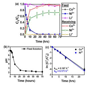
Fig. 6 (a) Transport of  ${\rm Co}^{2+}$  and  ${\rm Ni}^{2+}$  across an IEPIM in the feed and stripping solutions over time (b) plot of pH in the feed solution over time (c) kinetic plots of the transport of  ${\rm Co}^{2+}$  and  ${\rm Ni}^{2+}$  across the IEPIM in the feed solution.
