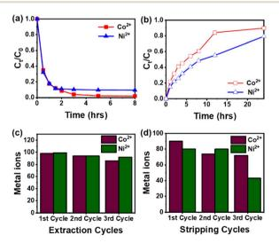
Fig. 3 (a) Extraction of Co<sup>2+</sup> and Ni<sup>2+</sup> into IEPIM in the feed solutions. (b) Stripping of Co<sup>2+</sup> and Ni<sup>2+</sup> from IEPIM in the stripping solutions. Three cycles of (c) extraction of Co<sup>2+</sup> and Ni<sup>2+</sup> into IEPIM and (d) stripping Co<sup>2+</sup> and Ni<sup>2+</sup> from IEPIM.
