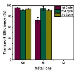
Fig. 8 Transport efficiency of 3 transport cycles. Feed solution: 100 mL of 0.1 mM Li<sup>+</sup>, Co<sup>2+</sup>, and Ni<sup>2+</sup>. Receiving solution: 2 M HCl. Membrane composition 50% wt PVDF-co-HFP and 30% wt Cyanex 301 and 20% wt [C<sub>8</sub>mim][NTf<sub>2</sub>]
