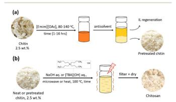
Fig. 3 (a) Ionic liquid pretreatment of chitin in [Emim][OAc] at different temperatures and time and (b) deacetylation of chitin into chitosan under various conditions.
