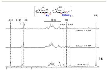
Fig. 7 <sup>1</sup>H NMR analysis gave structural information and the degree of deacetylation in chitin/chitosan samples.
