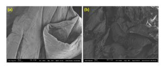
Fig. 5 SEM imaging (at  $200 \times$  magnification) illustrates chitin being more amorphous during IL pretreatment: (a) non-pretreated and (b) IL-pretreated at  $120 \, ^{\circ}\text{C}$ , 1 hour.
