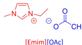
Fig. 2 Structure of 1-ethyl-3-methylimidazolium acetate, [Emim][OAc] IL.
