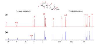
Fig. 6 Recovery of [Emim][OAc] IL was confirmed by spectroscopic data (<sup>1</sup>H and <sup>13</sup>C NMR) with (a) fresh IL and (b) recovered IL.
