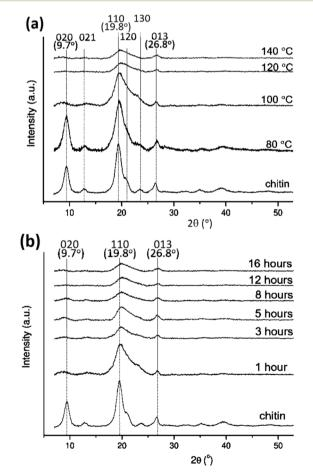
Fig. 4 XRD shows a decrease of chitin crystallinity when treated with [Emim][OAc] IL over (a) temperatures (80-140 °C, 1 hour) and (b) time (1-16 hours, 100 °C).
