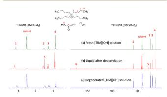
Fig. 11 Regeneration of [TBA][OH] was confirmed by  $^1\mathrm{H}$  and  $^{13}\mathrm{C}$  NMR analysis of (a) fresh solution, (b) liquid after the reaction, and (c) recovered solution.
