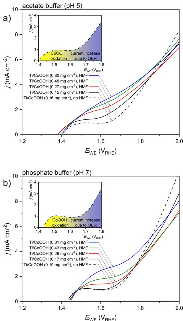
**Fig. 1** Linear sweep voltammograms of Ti/CoOOH electrodes with different catalyst loadings in the presence of 20 mM HMF (straight lines) (a) in acetate buffer – pH 5 and (b) in phosphate buffer – pH 7. Reference measurements without HMF (black dashed lines) are provided for the lowest catalyst loading. The inset figures schematically illustrate the transition from the CoOOH oxidation to the OER region in the respective electrolyte in the absence of HMF. The scan rate was 10 mV s<sup>-1</sup>.
