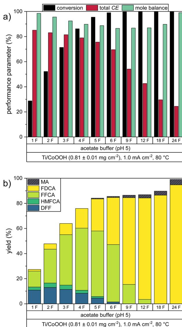
Fig. 5 Performance parameters of a HMF oxidation under optimized conditions (20 mM HMF in acetate buffer (pH 5), 80 °C,  $m_{\text{CoOOH}} = 0.81 \pm 0.01 \text{ mg cm}^{-2}$ ): (a) HMF conversion, total Coulomb efficiency, mole balance, remaining percentage of CoOOH and (b) product yields.
