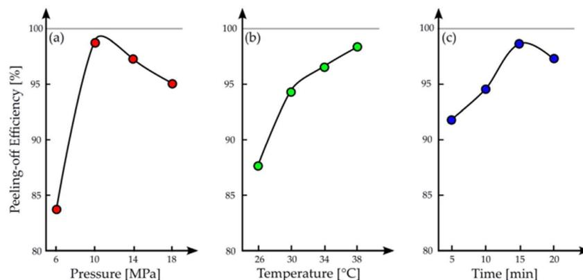
Fig. 10 Effect of (a) pressure, (b) temperature and (c) time on the exfoliation efficiency with scCO<sub>2</sub>. All graphics adapted from the work of Mu *et al.*<sup>74</sup> with permission from John Wiley and Sons.
