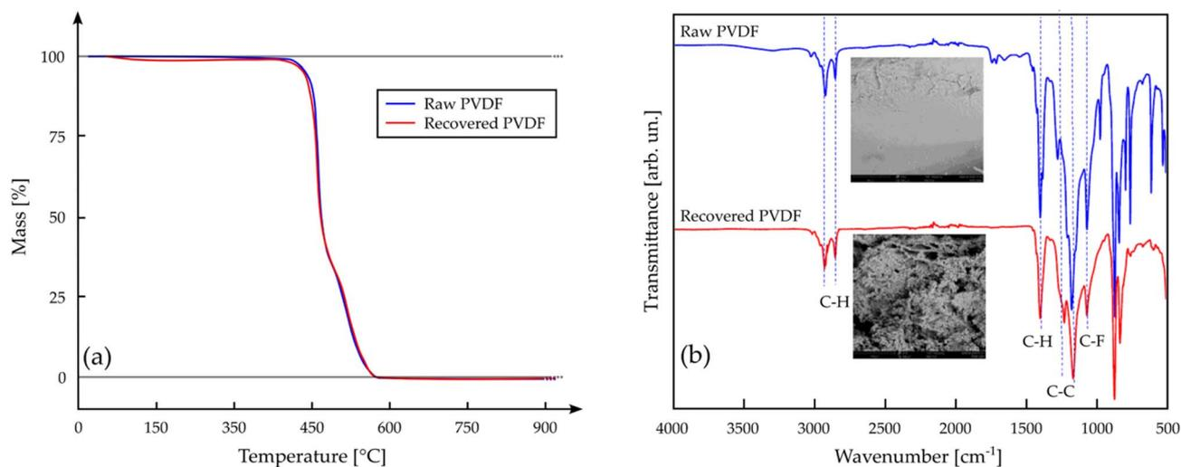
Fig. 9 Characterization of the PVDF recovered by Fu *et al.* (red plots) and comparison with raw PVDF (blue plots) as a reference by means of (a) TGA and (b) FT-IR analyses (adapted from ref. 122. Y. Fu, J. Schuster, M. Petranikova and B. Ebin, *Resour., Conserv. Recycl.*, 2021, **172**, 105666. No permission required. License: CC BY 4.0, Elsevier).
