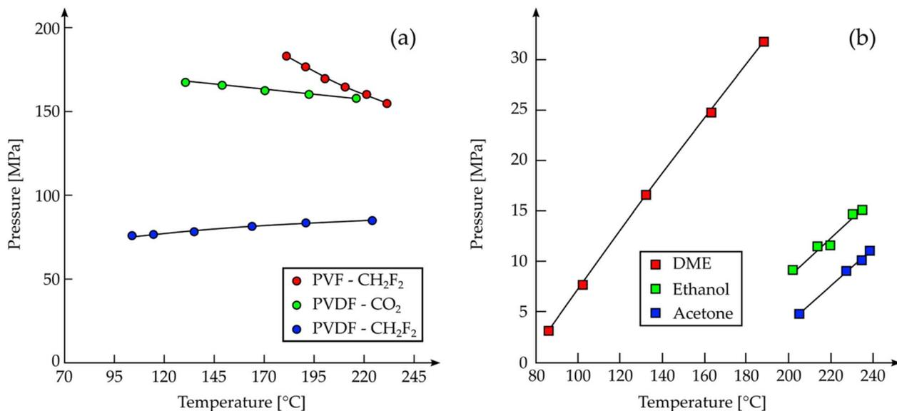
Fig. 7 (a) Cloud points of PVF in CH<sub>2</sub>F<sub>2</sub> (red) and PVDF in CO<sub>2</sub> (green) and in CH<sub>2</sub>F<sub>2</sub> (blue); (b) cloud points of PVDF in CO<sub>2</sub> with dimethyl ether, DME (red), ethanol (green) and acetone (blue) as co-solvents. All graphics adapted with permission of J. S. Lim and M. A. McHugh, *J. Phys. Chem. B*, 1999, 103, 2818. Copyright (1999) American Chemical Society.
