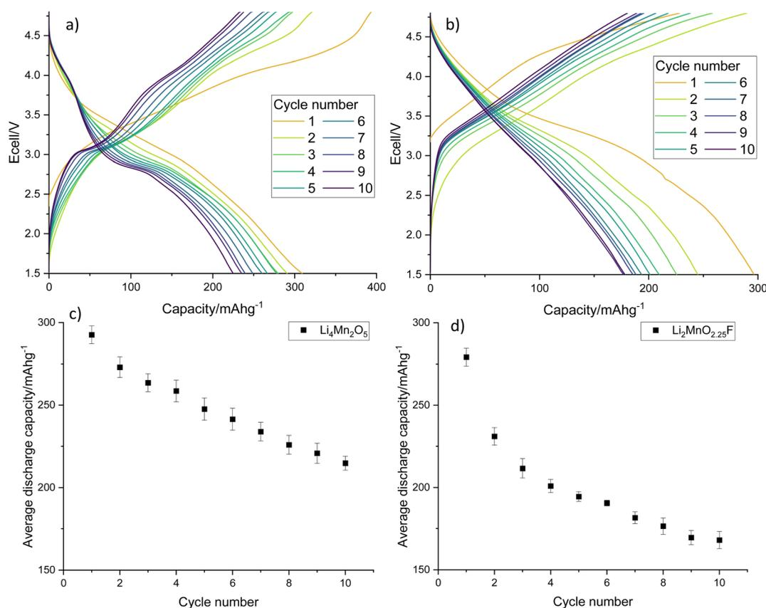
**Fig. 10** Galvanostatic charge–discharge profiles for (a)  $\text{Li}_4\text{Mn}_2\text{O}_5$  and (b)  $\text{Li}_2\text{MnO}_{2.25}\text{F}$  and average gravimetric discharge capacity against cycle number for (c)  $\text{Li}_4\text{Mn}_2\text{O}_5$  and (d)  $\text{Li}_2\text{MnO}_{2.25}\text{F}$ . Cells were cycled at  $10 \text{ mAg}^{-1}$  between 1.5–4.8 V.
