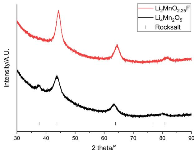
Fig. 9 XRD patterns of  $\text{Li}_4\text{Mn}_2\text{O}_5$  (black) and  $\text{Li}_2\text{MnO}_{2.25}\text{F}$  (red) made from recovered LMO (Cu  $K\alpha$ ). Tick marks correspond to a rocksalt phase.
