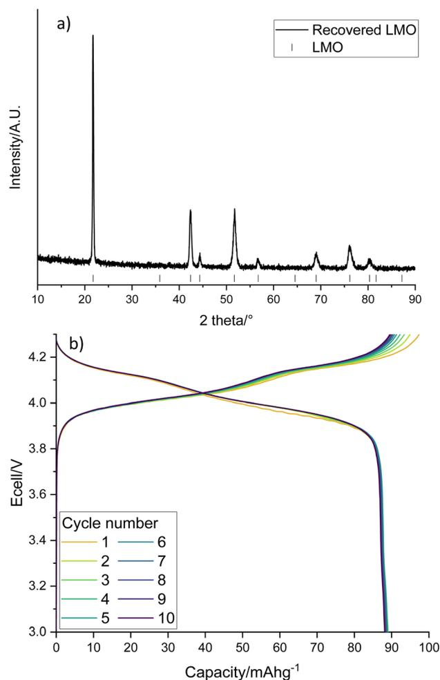
**Fig. 6** (a) XRD pattern of recovered LMO (Co K $\alpha$ ) with tick marks correspond to LMO and (b) galvanostatic charge–discharge profile of recovered LMO when cycled at 10 mAg<sup>-1</sup> between 3–4.3 V.
