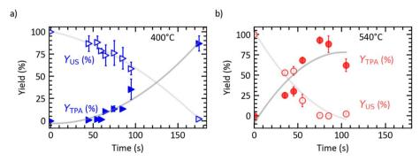
Fig. 2 Effects of batch holding time on yields of TPA and undissolved solids from PET fast hydrolysis at  $T_{SP}$  of (a) 400 °C and (b) 540 °C ( $m_{PET}/m_w = 1/10$ ). The grey lines are a guide to the eyes.
