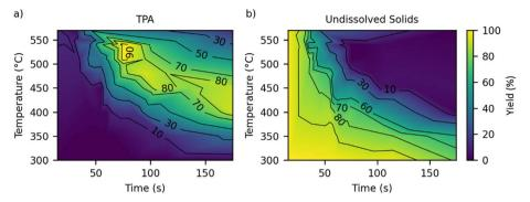
Fig. 3 Contour plot illustrating effects of set point temperature and batch holding time on (a) TPA yield and (b) yield of undissolved solids from fast hydrolysis of PET  $(m_{PET}/m_w = 1/10)$ .
