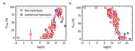
Fig. 4 (a) TPA molar yield and (b) yield of undissolved solids vs. log of the severity index for isothermal hydrolysis<sup>12</sup> ("filled circles") and fast hydrolysis ("empty squares") of post-consumer PET.
