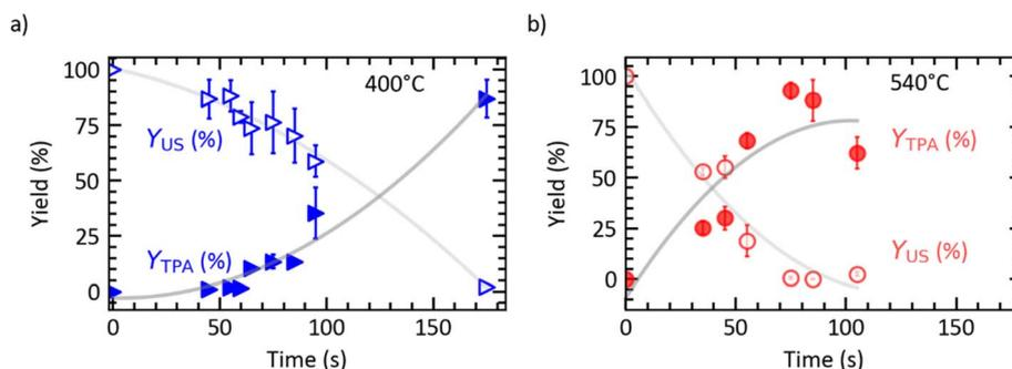
Fig. 2 Effects of batch holding time on yields of TPA and undissolved solids from PET fast hydrolysis at  $T_{SP}$  of (a) 400 °C and (b) 540 °C ( $m_{PET}/m_w = 1/10$ ). The grey lines are a guide to the eyes.
