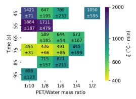
Fig. 6 Effect of batch holding time and  $m_{\rm PET}/m_{\rm w}$  on the environmental energy impact metric from fast hydrolysis of post-consumer PET at  $T_{SP} = 510 \,^{\circ}\text{C}$
