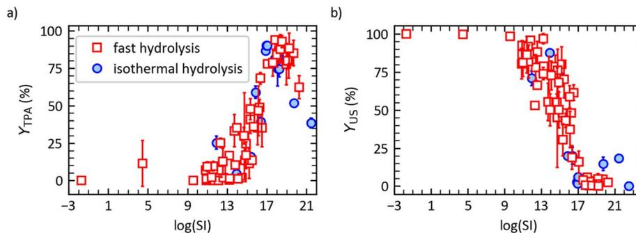
Fig. 4 (a) TPA molar yield and (b) yield of undissolved solids vs. log of the severity index for isothermal hydrolysis<sup>12</sup> ("filled circles") and fast hydrolysis ("empty squares") of post-consumer PET.
