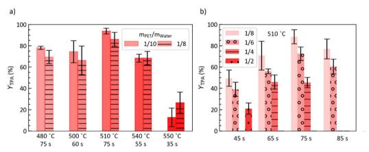
Fig. 5 TPA yield from fast hydrolysis of post-consumer PET for (a)  $m_{\rm PET}/m_{\rm w}=1/10$  and 1/8 at  $T_{\rm SP}$  and t indicated, and (b) different  $m_{\rm PET}/m_{\rm w}$  and t at  $T_{\rm SP}=510$  °C.
