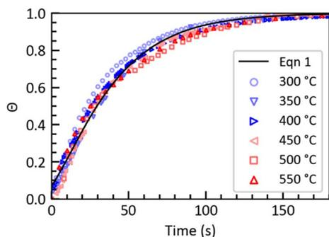
Fig. 1 Measured reactor temperature profiles (discrete points) at different  $T_{SP}$  and calculated via eqn (1) (solid line).
