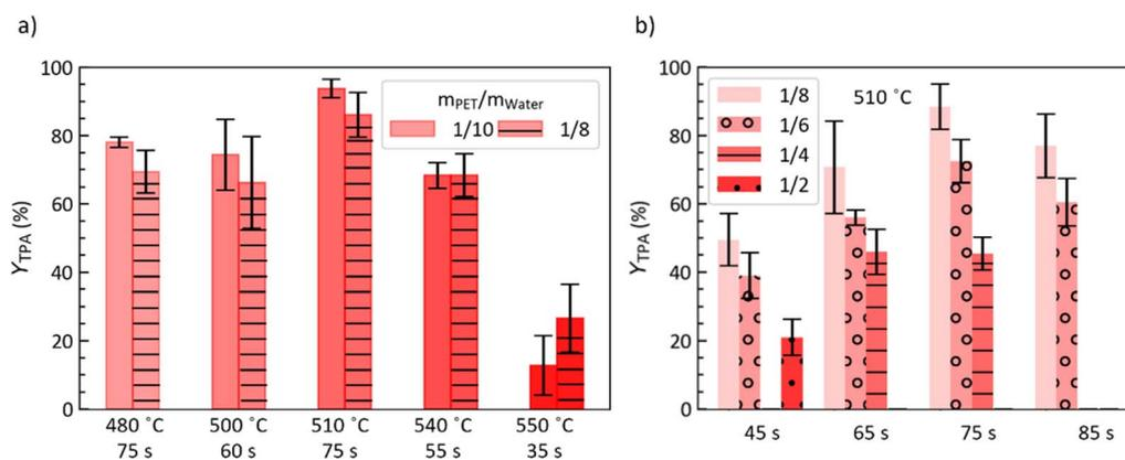
Fig. 5 TPA yield from fast hydrolysis of post-consumer PET for (a)  $m_{\text{PET}}/m_w = 1/10$  and  $1/8$  at  $T_{\text{SP}}$  and  $t$  indicated, and (b) different  $m_{\text{PET}}/m_w$  and  $t$  at  $T_{\text{SP}} = 510$  °C.
