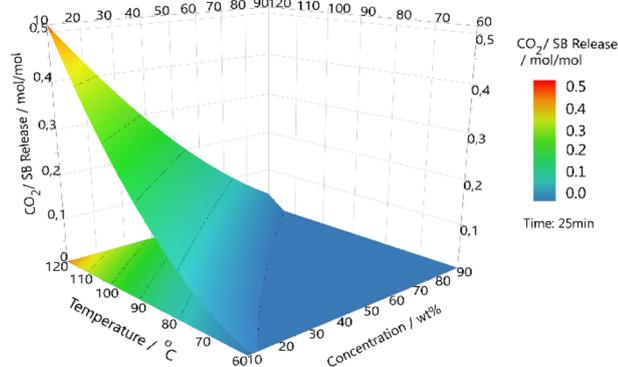
Fig. 3 Design of experiment surface plot of TBN in butyl acetate after 25 minutes of CO<sub>2</sub> exposure.
