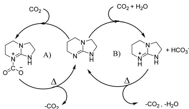
Fig. 1 Absorption schematic of CO<sub>2</sub> using TBN: (A) without water leading to the formation of zwitterions and (B) with the presence of water forming bicarbonate.
