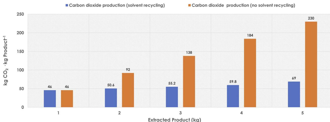
Fig. 2 Assessment of the  $CO_2$  production during an extractive downstream from a DES media, using an organic solvent, and reusing it for several cycles. Data assumed for extracting 10 L of DES, to produce 1 kg product at 100 g substrate per  $L_{DES}$ , and that two-fold volume of extractive solvent is used (20 L). 10% of solvent loss is assumed between each cycle.
