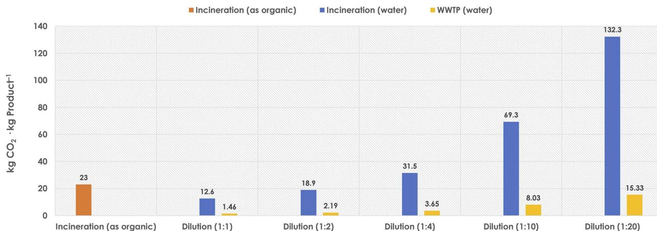
Fig. 4 Obtained TCRs (kg CO<sub>2</sub> per kg product) when treating 10 L DES as expended reaction media (needed to produce 1 kg product at 100 g substrate per L<sub>DES</sub>), and following different options such as organic incineration, or different aqueous dilution ratios and establishing water incineration or mild wastewater treatment (WWTP). Calculations based on TCR methods retrieved from literature.<sup>43,45,46</sup>
