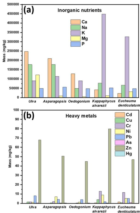
Fig. 7 Variation of (a) inorganic nutrients and (b) heavy metals present in biochar samples.
