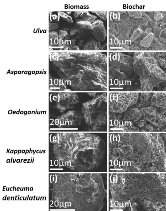
Fig. 2 SEM images of 5 macroalgal biomass and biochar samples: *Ulva* sp. (a) biomass, (b) biochar; *Asparagopsis* (c) biomass (d) biochar; *Oedogonium* sp. (e) biomass, (f) biochar; *Kappaphycus alvarezii* (g) biomass (h) biochar; *Eucheuma denticulatum* (i) biomass (j) biochar.
