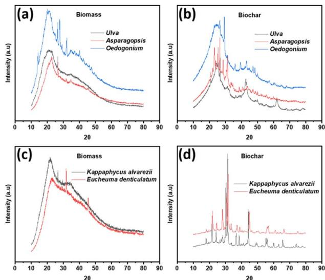
Fig. 4 X-ray diffraction patterns of (a) biomass (*Ulva* sp., *Asparagopsis* and *Oedogonium* sp.), (b) biochar (*Ulva* sp., *Asparagopsis* and *Oedogonium* sp.), (c) biomass (*Kappaphycus alvarezii* and *Eucheuma denticulatum*) and (d) biochar (*Kappaphycus alvarezii* and *Eucheuma denticulatum*).
