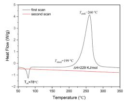
Fig. 2 DSC traces of M1 at a heating rate of 10 °C min<sup>-1</sup> in N<sub>2</sub>.
