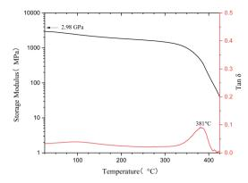
DMA curves of cured M1 at a heating rate of 5 °C min<sup>-1</sup> in N<sub>2</sub>.
