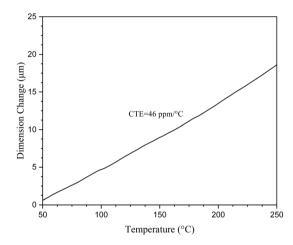
Fig. 6 CTE curve of cured M1 at a heating rate of 5 °C min<sup>-1</sup> in N<sub>2</sub>.
