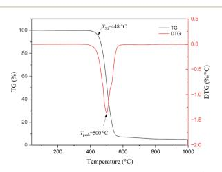
Fig. 4 TGA curve of cured M1 at a heating rate of 10 °C min<sup>-1</sup> in N<sub>2</sub>.
