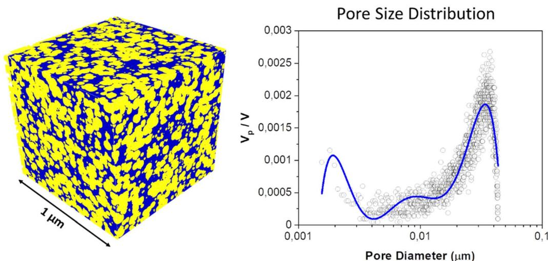
**Fig. 2** Left hand:  $1 \mu\text{m}^3$  cube of simulated C–S–H phases. The yellow color represents the C–S–H phases and the blue color represents the pores. Right hand: typical pore size distribution of C–S–H phases.
