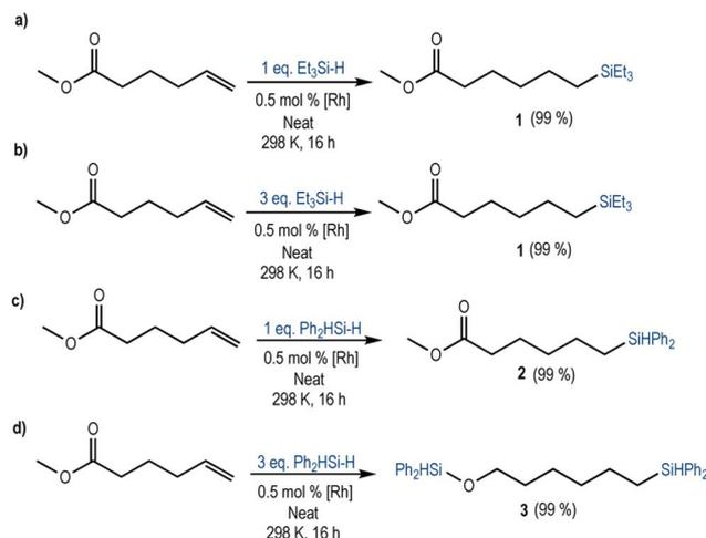
**Scheme 2** Reaction of methyl 5-hexenoate (0.25 mmol) with Et<sub>3</sub>SiH (a, 0.25 mmol; b, 0.75 mmol) and Ph<sub>2</sub>SiH<sub>2</sub> (c, 0.25 mmol; d, 0.75 mmol). Yields were calculated based on <sup>1</sup>H NMR (CDCl<sub>3</sub>) analysis using 1,2-dichloroethane (0.0625 mmol) as an internal standard.
