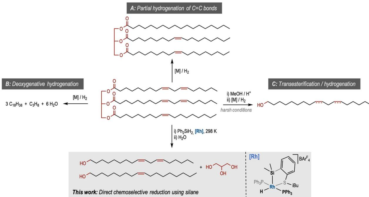
Fig. 1 Different pathways for the reduction of plant oils and the structure of the  $[\text{Rh}(\text{SiS}^i\text{Bu})]$  complex used in this study.
