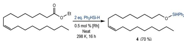
**Scheme 3** Catalytic hydrosilylation of ethyl oleate (0.25 mmol) using 0.50 mmol of Ph<sub>2</sub>SiH<sub>2</sub>. Yields were calculated based on <sup>1</sup>H NMR (CDCl<sub>3</sub>) analysis using 1,2-dichloroethane (0.065 mmol) as an internal standard.
