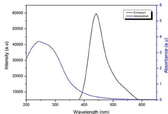
Fig. 3 UV absorbance and fluorescence emission of CD water solution ( $\lambda_{\text{max exc}} = 370 \text{ nm}$ ).
