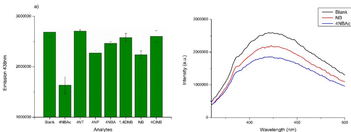
Fig. 5 (a) PL emissions at  $\lambda_{\max}$  of CD aqueous solution treated with different nitro compounds; (b) comparative analysis of PL emission spectra in CD solution compared to NB and NBAC solutions.
