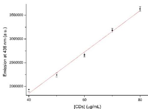
Fig. 4 Calibration curve of CDs's fluorescence emission.
