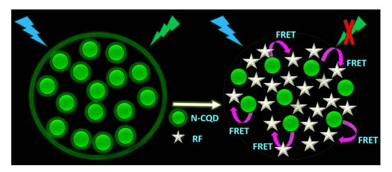
Scheme 2 Schematic representation of the FRET mechanism between N-CQDs and RF leading to quenching of fluorescence emission from N-CQDs.
