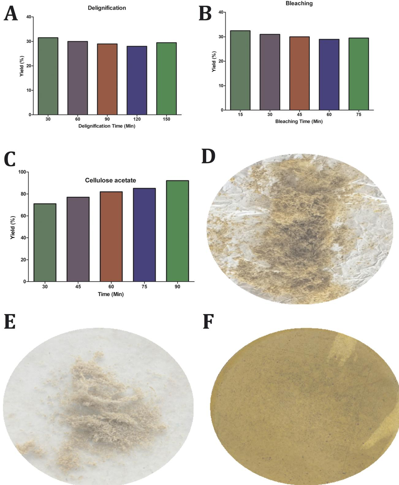
**Fig. 1** Cellulose Acetate Film preparation. (A) Incubation duration of *Musa acuminata* leaf extract for delignification, (B) incubation duration of the delignified sample for bleaching, (C) incubation duration for acetylation of the extracted cellulose, (D) extracted cellulose sample from *Musa acuminata*, (E) acetylated cellulose sample and (F) cellulose acetate film.
