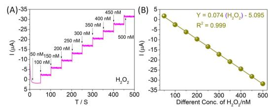
Fig. 8 Chrono-program in various concentrations of  $H_2O_2$  (50–500 nM) at (A) CTH/MWCNT-modified GC electrode in PBS (pH 7) electrolyte. (B) Linear graph of various concentrations of  $H_2O_2$  vs. various reduction peaks currents: at the applied potential of 400 mV s<sup>-1</sup>.
