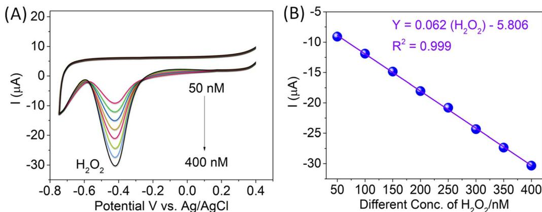
Fig. 6 Cyclic voltammogram in various concentrations of  $\text{H}_2\text{O}_2$  (50–400 nM) at (A) the CTH-modified GC electrode with composite MWCNTs in PBS (pH 7) electrolyte. (B) Linear graph of various concentrations of  $\text{H}_2\text{O}_2$  vs. various reduction peak currents: scan rate:  $50 \text{ mV s}^{-1}$ .
