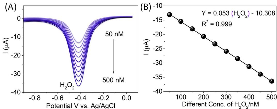
Fig. 7 Differential pulse voltammogram in various concentrations of  $\text{H}_2\text{O}_2$  (50–500 nM) at (A) CTH/MWCNT-modified GC electrode in PBS (pH 7) electrolyte. (B) Linear graph of various concentrations of  $\text{H}_2\text{O}_2$  vs. various reduction peaks current: scan rate  $50 \text{ mV s}^{-1}$ .
