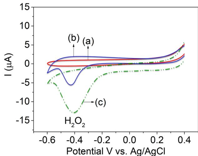
Fig. 5 Cyclic voltammogram in 150 nM  $\text{H}_2\text{O}_2$  at (a) the bare GC electrode; (b) CTH-modified GC electrode and (c) CTH-modified GC electrode with composite MWCNTs in PBS (pH 7) electrolyte. Scan rate:  $50 \text{ mV s}^{-1}$ .
