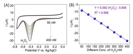
Fig. 6 Cyclic voltammogram in various concentrations of  $H_2O_2$  (50–400 nM) at (A) the CTH-modified GC electrode with composite MWCNTs in PBS (pH 7) electrolyte. (B) Linear graph of various concentrations of  $H_2O_2$  vs. various reduction peak currents: scan rate: 50 mV s<sup>-1</sup>.
