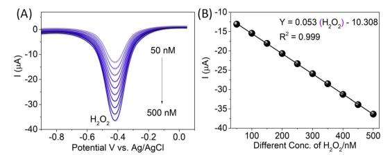
Fig. 7 Differential pulse voltammogram in various concentrations of  $H_2O_2$  (50–500 nM) at (A) CTH/MWCNT-modified GC electrode in PBS (pH 7) electrolyte. (B) Linear graph of various concentrations of  $H_2O_2$  vs. various reduction peaks current: scan rate 50 mV s<sup>-1</sup>.
