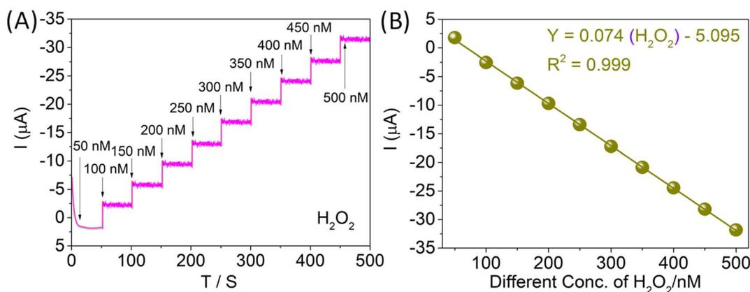
Fig. 8 Chrono-program in various concentrations of  $\text{H}_2\text{O}_2$  (50–500 nM) at (A) CTH/MWCNT-modified GC electrode in PBS (pH 7) electrolyte. (B) Linear graph of various concentrations of  $\text{H}_2\text{O}_2$  vs. various reduction peaks currents: at the applied potential of  $400 \text{ mV s}^{-1}$ .
