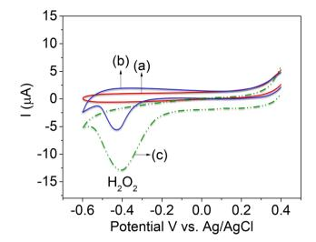
Fig. 5 Cyclic voltammogram in 150 nM H<sub>2</sub>O<sub>2</sub> at (a) the bare GC electrode; (b) CTH-modified GC electrode and (c) CTH-modified GC electrode with composite MWCNTs in PBS (pH 7) electrolyte. Scan rate: 50 mV s<sup>-1</sup>.
