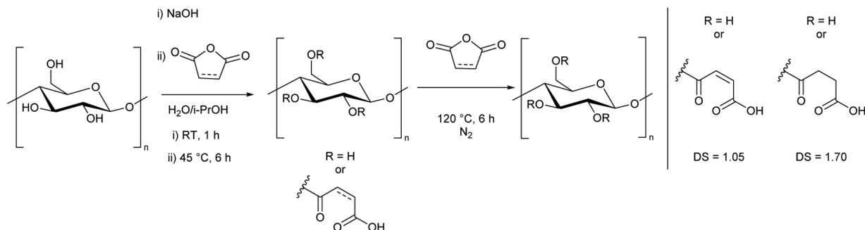
**Scheme 3** Alternate syntheses of modified cellulose where 1,3-propane sultone is replaced with (top) maleic or succinic anhydride, or (bottom) 1,4-butane sultone. These modified celluloses were not water-soluble.
