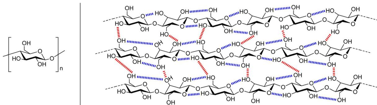
Fig. 1 A representation of the structure of cellulose. Left is the anhydroglucose unit (AGU) and right shows the inter- (red) and intramolecular (blue) hydrogen bonds.
