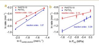
Fig. 3 Reaction order of (a) vanillyl alcohol and (b)  $H_2$  over the Pd/ETS-10 and Pd/TiO<sub>2</sub> catalysts. Reaction conditions for vanillyl alcohol reaction order: 200–350 mg of vanillyl alcohol, 1 mg of catalyst, 10 g of  $H_2$ O, 1 MPa of  $H_2$ , 120 °C, 0.17 h. Reaction conditions for  $H_2$  reaction order: 200 mg of vanillyl alcohol, 1 mg of catalyst, 10 g of  $H_2$ O, 0.2–1 MPa of  $H_2$ , total pressure at 1 MPa, balanced with  $H_2$ , 120 °C, 0.17 h.
