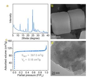
Fig. 1 (a) XRD pattern, (b) SEM image, (c) N<sub>2</sub>-sorption isotherms, and (d) TEM image of the Pd/ETS-10 sample.
