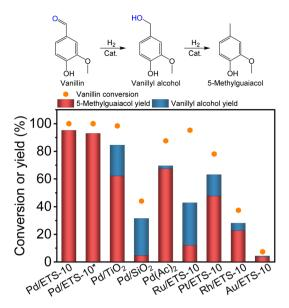
Fig. 2 Catalytic hydrodeoxygenation of vanillin over various catalysts. Typical reaction conditions: 1 g of vanillin, 0.2 g of catalyst, 50 g of H<sub>2</sub>O, 1 MPa of H<sub>2</sub>, 120 °C, 1.5 h. Reaction conditions for Pd/ETS-10\*: 152 mg of vanillin, 134.4 mg of catalyst, 10 g of  $H_2O$ , 2 MPa of  $H_2$ , 60 ° C, 5 h.
