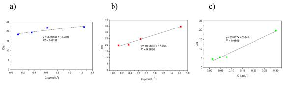
Fig. 11 Langmuir model of (a)  $Cr^{3+}$ , (b)  $Cd^{2+}$ , (c)  $Pb^{2+}$
