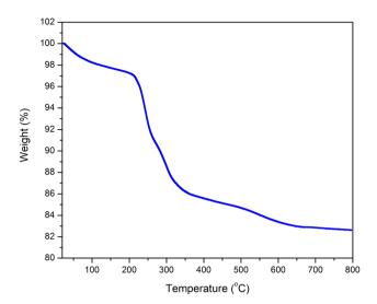
Fig. 4 Thermal gravimetric analysis diagram of DL1-SiO<sub>2</sub>.
