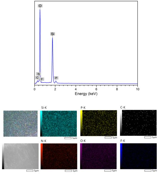
Fig. 5 EDX spectrum and SEM mapping of elemental distribution in DL1-SiO<sub>2</sub>.
