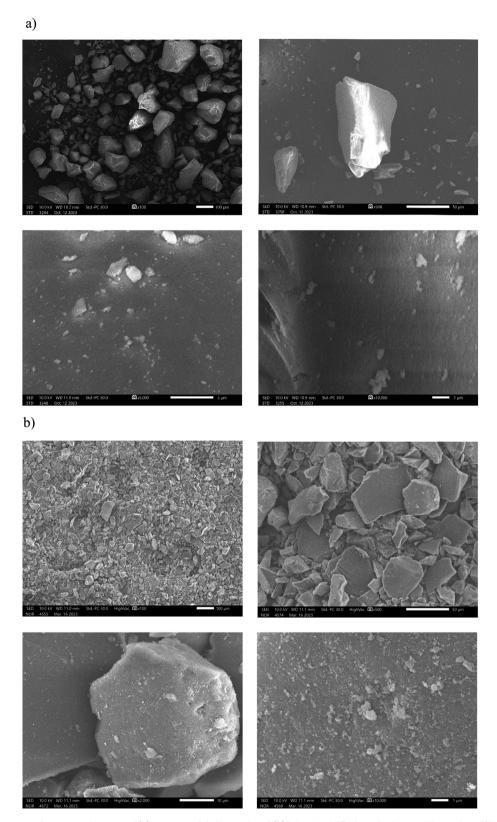
Fig. 6 Scanning electron microscopy images of (a) commercial silica gel and (b) ionic liquid DL1 grafted onto silica gel at different magnifications.
