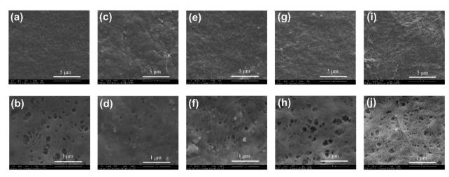
Fig. 5 SEM images (surface) of the (a and b) pristine BC, (c and d) 3% C0-BC-1 h, (e and f) 5% C8-BC-1 h, (g and h) 10% C12-BC-1 h, and (i and j) 15% C18-BC-1 h films at  $20\,000\times$  and  $100\,000\times$  magnification, respectively.
