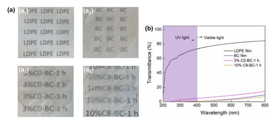
Fig. 9 (a) Photographs and (b) UV-vis spectra of the LDPE, pristine BC, 3% C0-BC-1 h, and 10% C8-BC-1 h films
