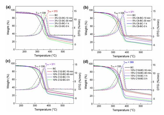
Fig. 11 Thermogravimetric analysis and DTG of the pristine BC and (a) 3% CO-BC, (b) 5% C8, (c) 10% C12, and (d) 15% C18-BC films at 10 min-3 h.
