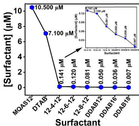
Fig. 10 Comparison plot illustrating the concentration of various investigated cationic surfactants where 50% ct-DNA compaction occurred in the presence of silica nanoparticles ( $\sim 100$  nm) systems in Tris-HCl buffer (pH = 7.4,  $\sim 10$  mM),  $1.5 \times 10^{-3}$  wt% silica nanoparticles. Inset: Better visualization of the differences in concentrations for some surfactants.
