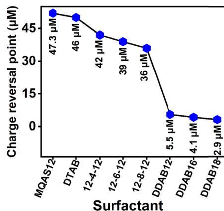
Fig. 2 Comparison plot illustrating the concentrations at which  $\zeta$  values become zero across various investigated cationic surfactants in the presence of silica nanoparticles ( $\sim 100$  nm) in Tris HCl buffer (pH = 7.4,  $\sim 10$  mM), where [surfactant] =  $2.5 \mu\text{M}$ ; [silica nanoparticles] =  $1.5 \times 10^{-3}$  wt%; [ct-DNA] =  $5.0 \mu\text{M}$ .
