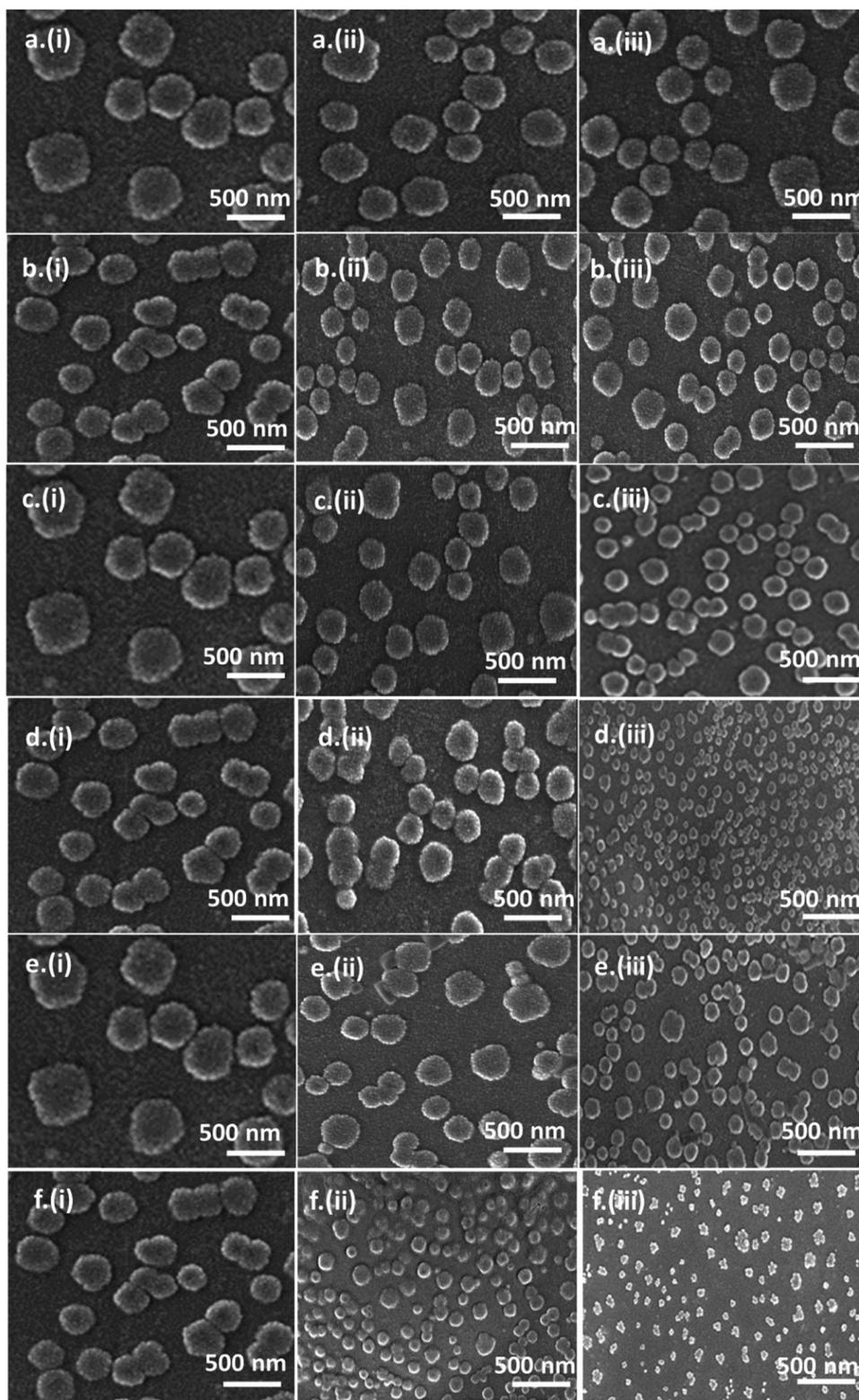
**Fig. 7** FE-SEM images elucidating the morphological changes in the ct-DNA structures compacted by MQAS12 (a) and (b), DDAB16 (c) and (d), and DDAB18 (e) and (f), at concentrations of (i) 0  $\mu\text{M}$ , (ii) 1.2  $\mu\text{M}$ , and (iii) 2.5  $\mu\text{M}$  in the absence [(a), (c) and (e)] and in the presence [(b), (d) and (f)] of  $\sim 100$  nm silica nanoparticles ( $1.5 \times 10^{-3}$  wt%) in Tris-HCl buffer (pH = 7.4,  $\sim 10$  mM). [ct-DNA] = 5.0  $\mu\text{M}$ .
