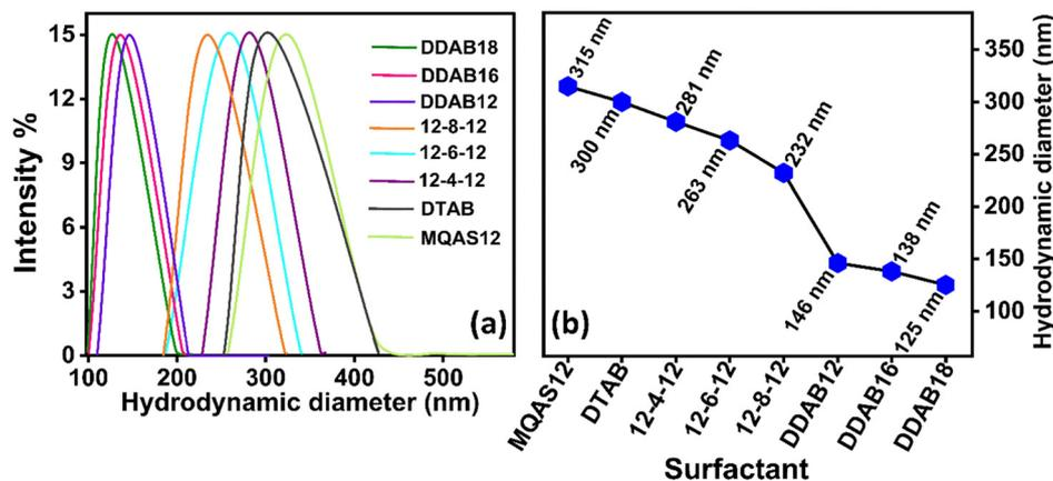
Fig. 8 Comparison plots illustrating the DLS size distribution (a) and hydrodynamic diameters (b) of various investigated cationic surfactants, ct-DNA, and silica nanoparticles ( $\sim 100$  nm) systems in Tris-HCl buffer (pH = 7.4,  $\sim 10$  mM) where [surfactant] =  $2.5 \mu\text{M}$ ;  $1.5 \times 10^{-3}$  wt% silica nanoparticles; [ct-DNA] =  $5.0 \mu\text{M}$ .
