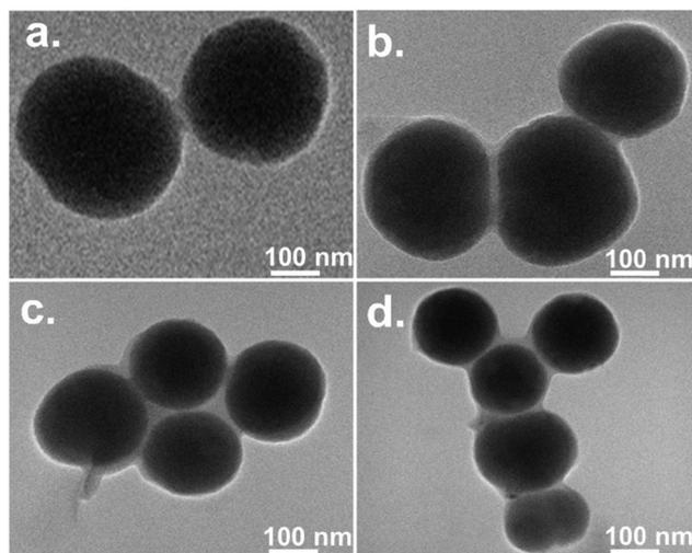
Fig. 6 TEM images of the ct-DNA structures compacted by 2.5  $\mu\text{M}$  of MQAS12 (a), DTAB (b), 12-6-12 (c), and DDAB18 (d) in the presence of  $\sim 100$  nm silica nanoparticles ( $1.5 \times 10^{-3}$  wt%) in Tris-HCl buffer (pH = 7.4,  $\sim 10$  mM), [ct-DNA] = 5.0  $\mu\text{M}$ .
