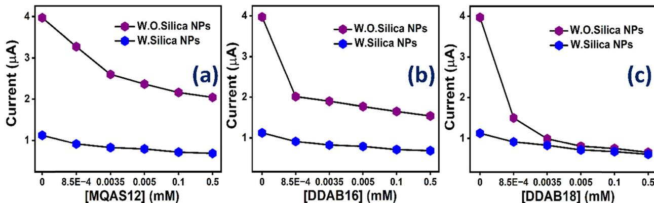
Fig. 3 Comparison plots of the anodic current taken at a particular potential *i.e.*, ~0.76 V for (a) MQAS12, (b) DDAB16, and (c) DDAB18 surfactants at different concentrations both in the presence and absence of silica nanoparticles ( $1.5 \times 10^{-3}$  wt%, ~100 nm) in Tris HCl buffer (pH = 7.4, ~10 mM); [ct-DNA] = 5.0  $\mu\text{M}$ . (W.O. = without; W = with).
