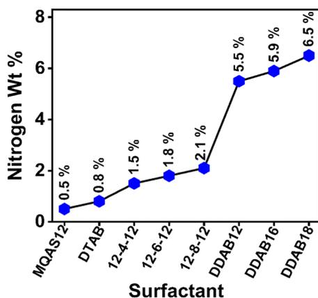
Fig. 1 Comparison plot illustrating nitrogen wt% across various investigated cationic surfactants in the presence of silica nanoparticles in Tris HCl buffer (pH = 7.4,  $\sim 10$  mM), where [surfactant] =  $2.5 \mu\text{M}$ ;  $1.5 \times 10^{-3}$  wt% silica nanoparticles ( $\sim 100$  nm); [ct-DNA] =  $5.0 \mu\text{M}$ .
