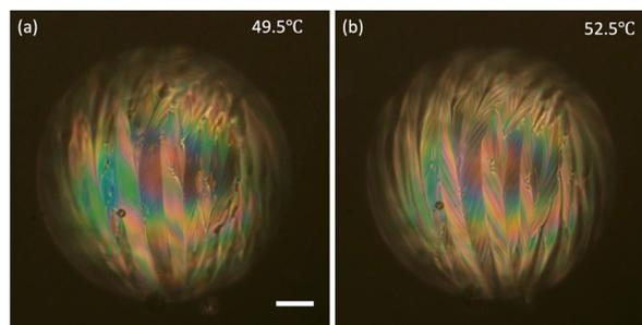
**Fig. 6** POM images of a shell on heating from SmC to SmA (still images from Supporting Video 2, ESI†). In the SmC phase (a) the secondary modulation is absent but on heating to the SmA phase (b) it reappears. However, the number of lunes and their width remain almost the same as in SmC even after the transition. Scale bar represents 50  $\mu\text{m}$ .
