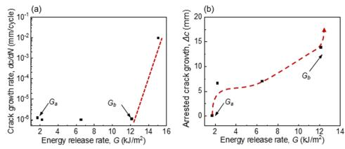
Fig. 9 Crack growth in a knit-PCU composite. (a) The crack growth rate dc/dN as a function of the energy release rate G. (b) The arrested crack growth after 20 000 cycles as a function of the energy release rate G.
