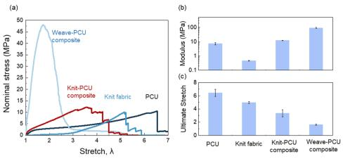
Fig. 4 (a) Stress-stretch curves of four materials: PCU, knit fabric, knit-PCU composite, and weave-PCU composite. (b) Moduli and (c) ultimate stretches of the three materials
