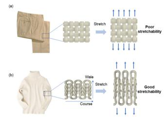
Fig. 1 (a) A woven fabric is nearly incompressible. (b) A knitted fabric is highly stretchable.
