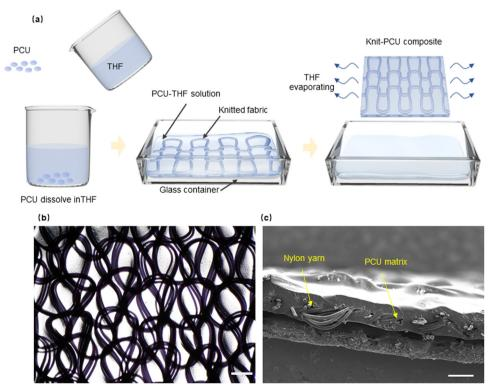
Fig. 3 (a) Fabrication of a knit-PCU composite. (b) Image of the composite in an optical microscope. Scale bar is 200 µm. (c) Image of the composite in a scanning electron microscope. Scale bar is 200 µm.
