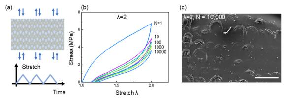
Fig. 7 A knit-PCU composite without precut crack under cyclic stretch. (a) Schematic of the cyclic test of the sample without precut. (b) Cyclic stressstretch curve. (c) Scanning electron microscope image of the composite after 10 000 cycles. The scale bar is 500 µm.
