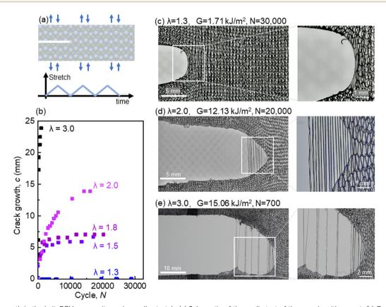
Fig. 8 Crack growth in the knit-PCU composite under cyclic stretch. (a) Schematic of the cyclic test of the sample with precut. (b) Crack growth as a function of the cycle number N. (c) Under a low amplitude of stretch,  $\lambda = 1.3$ , the crack does not grow. (d) Under an intermediate amplitude of stretch,  $\lambda=2.0$ , the crack grows and arrests. (e) Under a high amplitude of stretch,  $\lambda=3.0$ , the crack propagates continuously
