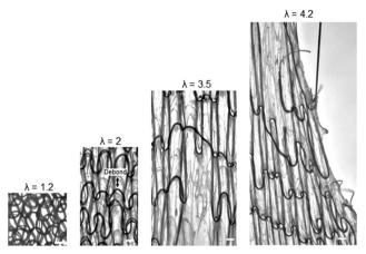
Snapshots of a knit-PCU composite stretched under an optical microscope. Scale bars are 200 µm.
