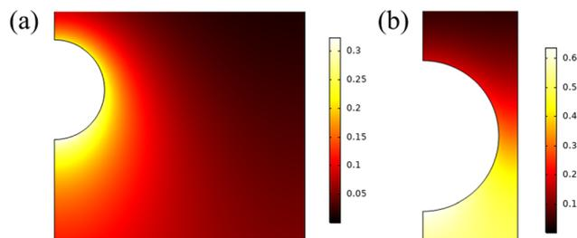
Fig. 9 Non-dimensional solute concentration around the particle, when suspended in a shear thinning fluid with  $Cu = 30$ ,  $n = 0.5$ ,  $\beta = 0.01$  for (a)  $\kappa = 0.2$  and (b)  $\kappa = 0.8$ . The solute concentration gradient for the latter case is clearly larger. The surface plots are shown for  $Pe = 10$ .
