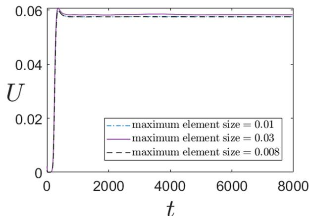
Fig. 10 Transient variation of axial phoretic velocity at  $Pe = 10$  for different maximum element sizes. The results shown above correspond to the particle suspended in a Carreau fluid with  $\beta = 0.01$ ,  $Cu = 30$ , and  $n = 0.25$ .
