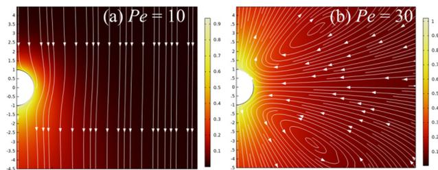
Fig. 3 Surface plot showing the variation of the solute concentration around the particle for (a)  $Pe = 10$  and (b)  $Pe = 30$ . The figures also presents the streamlines. The latter clearly shows the absence of particle motion in the second case, whereas a non-uniform distribution in the first case suggesting the origin of a phoretic flow.
