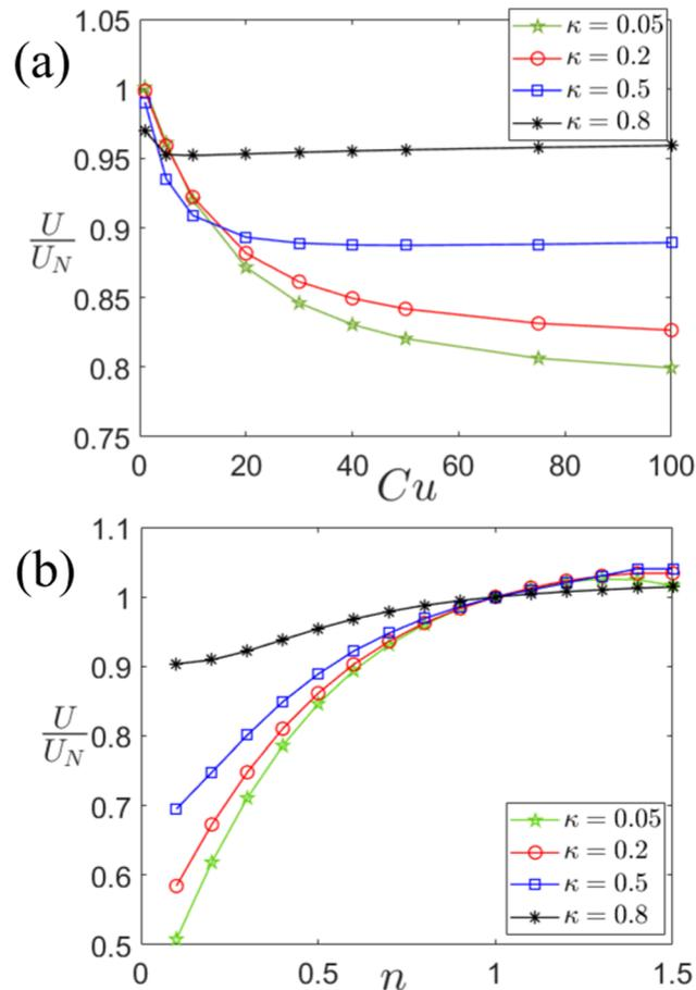
Fig. 8 Effect of confinement on the the axial phoretic velocity for  $\beta = 0.01$  at  $Pe = 10$ . (a) Variation of the normalized phoretic velocity of the isotropic active particle as a function of (a)  $Cu$  (with  $n = 0.5$ ) and (b)  $n$  (with  $Cu = 30$ ) for different values of  $\kappa$  ( $= 0.05, 0.2, 0.5, 0.8$ ).
