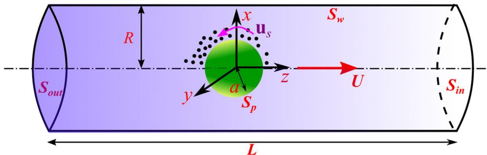
Fig. 1 A schematic of the physical system consisting of a particle of radius  $a$  suspended in a cylindrical microchannel of radius  $R$  and length  $L$ .  $U$  is the axial velocity of the particle which is due to the generation of slip velocity ( $\mathbf{u}_s$ ) at the particle surface ( $S_p$ ). The black dots denote the solutes generated as a result of the chemical reaction at the particle surface. The surface of the microchannel ( $S_w$ ) is considered as inert.
