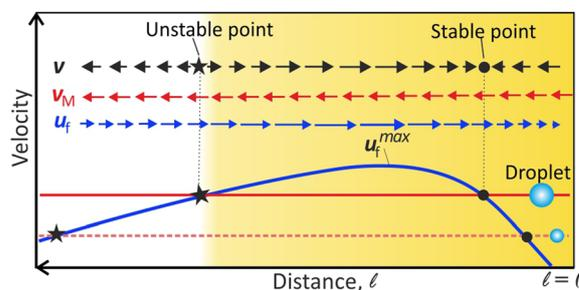
Fig. 3 Illustrated velocities of background convective flow ( $\mathbf{u}_f$ ; blue lines) and microdroplets ( $\mathbf{v}_M$ ; red lines). Unstable (★) and stable (●) equilibrium points are formed at  $\mathbf{v}_M + \mathbf{u}_f = 0$ . Arrows indicate velocity magnitude and direction for the large droplet. When the small droplet enlarges, its (dashed line)  $\mathbf{v}_M$  increases (solid line) resulting in smaller extent of the stable equilibrium region (highlighted yellow).
