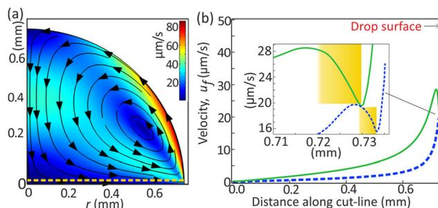
Fig. 2 (a) The simulated large Marangoni recirculating flow inside the drop. (b) The magnitude of the flow along the dashed cut-line drawn in (a) at two different heights  $z = 3$  (dashed line) &  $10 \mu\text{m}$  from the substrate. The region of drag force producing stepwise motion is highlighted in the inset.
