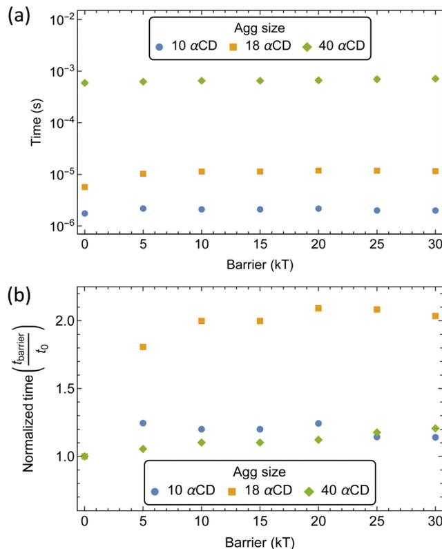
Fig. 10 Mean first passage time (MFPT) of aggregate formation along the mono-functionalized PEG<sub>5k</sub> backbone with increasing threading barriers. (a) Total assembling times at each barrier. (b) Normalized aggregation times relative to the time required for an unfunctionalized PEG.
