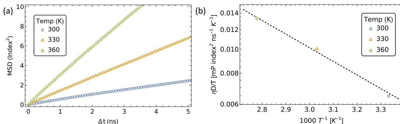
Fig. 7 Intrachain diffusion of  $\alpha$ CDs in a rPR. (a) MSD of  $\alpha$ CDs at different temperatures. (b) Diffusion coefficient versus temperature to determine the barrier to jumping ( $\Delta G_{\text{slide}}$ ) and frequency factor ( $A$ ).
