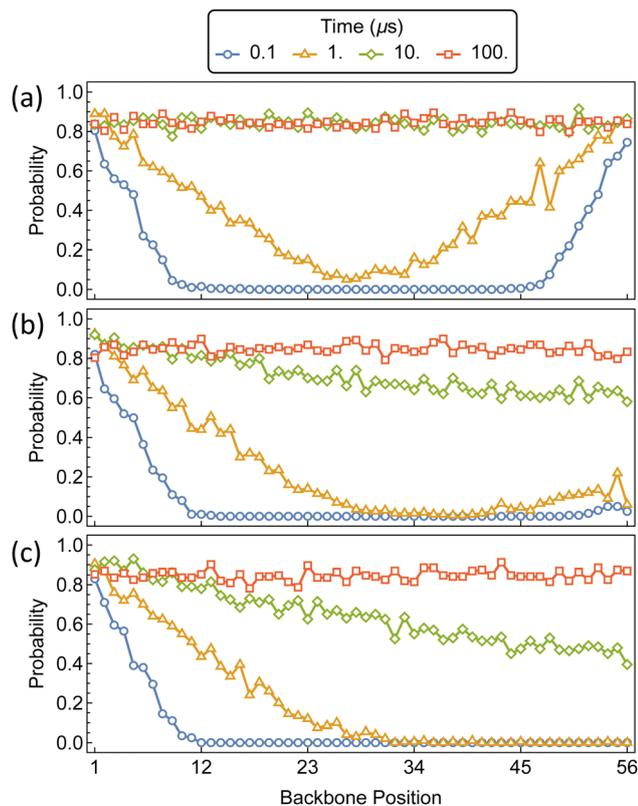
Fig. 9 Probability distributions of  $\alpha$ CDs migration along a bare PEG<sub>5k</sub> backbone (a) and monofunctionalized PEG<sub>5k</sub> with a threading barrier of 5 kT (b) and 10 kT (c) located at position 56.
