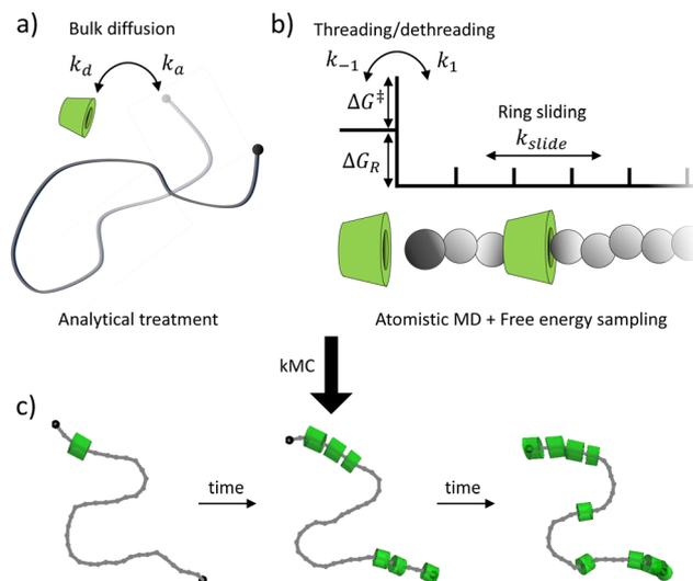
Fig. 1 Schematic illustration of the multi-scale kinetic model for PSR assembly. (a) Analytical treatment of the bulk diffusion of reactants in solution. (b) Atomistic molecular dynamics of backbone diffusion, and free energy sampling of the threading and dethreading process. (c) kMC for predicting the time-dependent PSR assembly.
