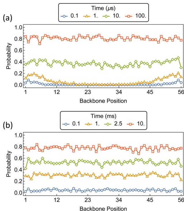
Fig. 11 Probability distributions of  $\alpha$ CDs migration along a bifunctionalized PEG<sub>5k</sub> backbone with barriers at position 1 and 56. Barrier sizes are (a) 5 kT, and (b) 10 kT.
