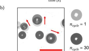
Fig. 12 Effect of the periodic pressure treatment on the bubble relative position. Representative parts of (a) periodic pressure treatment (red), bubble radius evolution (black), interbubble distance (blue). (b) Compar ison of bubble positions after 30 cycle. Scale bar is 1000  $\mu m$ .
