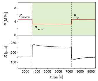
Fig. 7 Effect of bubble pressure on bubble growth dynamics. Imposed pressure history (red) and bubble radius evolution (black). The bubble inflate or deflate when the pressure is reduced or increased.
