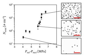
Fig. 2 Bubble number density vs. pressure reduction at a fixed  $P_{\text{sat}}$  = 8.1 MPa. Scale bar is 1000 μm.
