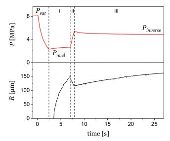
Fig. 4 Inverse pressure quenching treatment: imposed pressure history (red) and bubble radius evolution (black); three different growth dynamics regimes corresponding to the pressure variation can be identified: first bubble growth (I), size reduction caused by the pressure increase (II), second bubble growth (III).
