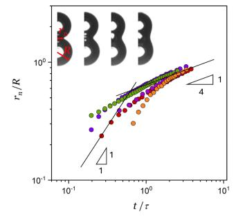
Fig. 11 Coalescence of two bubbles of almost the same size in a PP/N<sub>2</sub> system, at P = 4.0 MPa. Evolution of the normalized neck radius  $(r_n/R)$ against the dimensionless time  $(t/\tau)$ .
