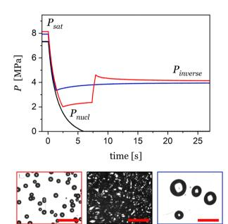
Fig. 5 Pressure history of the inverse pressure quench treatment (red), comparison with two simple pressure quench treatments (black and blue) and images of the sample at a t = 20 s. Scale bar is 1000  $\mu m$ .
