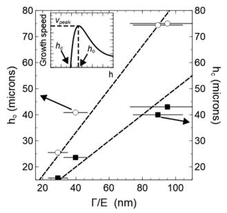
**Fig. 7**  $\Gamma/E$  dependence of the thickness corresponding to the peak growth speed,  $h_0$  (left axis), and the critical thickness,  $h_c$  (right axis), below which blisters do not grow for solvent swollen PDMS films. The dashed lines are linear fits to the  $h_c$  and  $h_0$  data. The diagram/plot given as an inset shows how  $h_0$ ,  $h_c$  and  $v_{\rm peak}$  are defined.
