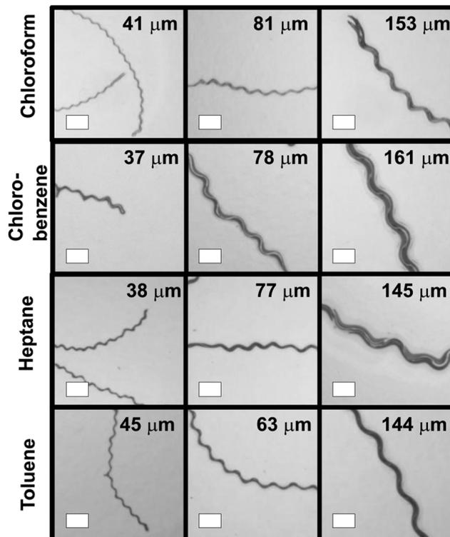
**Fig. 2** Images showing large-slope folded telephone cord blisters formed on 10 : 1 (resin : crosslinker) PDMS films during swelling with chlorobenzene, chloroform, heptane and toluene. All of the blisters are imaged from above. The scale bar represents 1 mm in each image. Thickness values of the PDMS films are given as insets in each panel.
