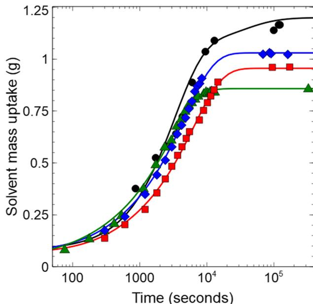
Fig. 3 Solvent mass uptake of 20 mm diameter, 3 mm thick, 10:1 (resin:crosslinker) PDMS disks as a function of time for chlorobenzene (red squares), chloroform (black circles), heptane (green triangles) and toluene (blue diamonds). Solid lines are fits to the first three terms of the expansion in eqn (1). Values obtained for the diffusion coefficient,  $D$ , are summarised in Table 1.
