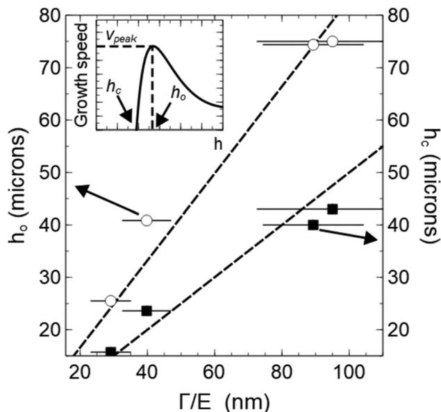
Fig. 7  $\Gamma/E$  dependence of the thickness corresponding to the peak growth speed,  $h_0$  (left axis), and the critical thickness,  $h_c$  (right axis), below which blisters do not grow for solvent swollen PDMS films. The dashed lines are linear fits to the  $h_c$  and  $h_0$  data. The diagram/plot given as an inset shows how  $h_0$ ,  $h_c$  and  $v_{\text{peak}}$  are defined.
