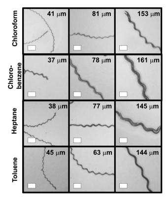
Fig. 2 Images showing large-slope folded telephone cord blisters formed on 10:1 (resin: crosslinker) PDMS films during swelling with chlorobenzene, chloroform, heptane and toluene. All of the blisters are imaged from above. The scale bar represents 1 mm in each image. Thickness values of the PDMS films are given as insets in each panel.
