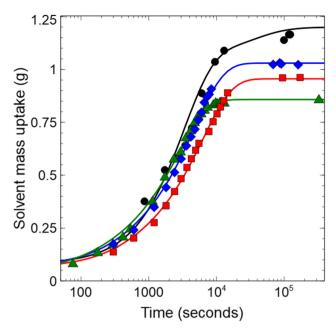
Fig. 3 Solvent mass uptake of 20 mm diameter, 3 mm thick, 10:1 (resin:crosslinker) PDMS disks as a function of time for chlorobenzene (red squares), chloroform (black circles), heptane (green triangles) and toluene (blue diamonds). Solid lines are fits to the first three terms of the expansion in eqn (1). Values obtained for the diffusion coefficient, *D*, are summarised in Table 1.
