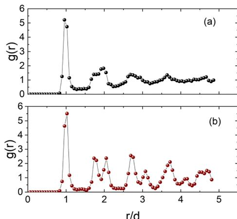
Fig. 11  $g(r)$  curves of the vibrated polystyrene beads in which the (a) glass-like state and (b) crystalline state can be observed.
