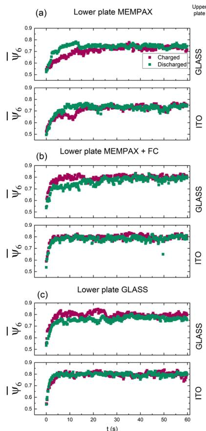
**Fig. 10** Comparison of the temporal evolution of the average of the sixth orientational order parameter between an initial condition of uncharged particles and plates and an initially charged condition for (a) MEMPAX, (b) MEMPAX + FC, and (c) glass as the bottom plate.
