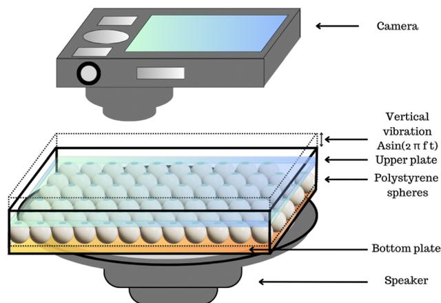
Fig. 1 A schematic representation of the experimental setup. The container is fixed to a speaker. The ensemble of particles is sandwiched by a bottom plate, which is attached to the square container, and an upper plate, which lies over the particles and moves freely. The container moves harmonically in the vertical direction, and top-view observations are recorded using a camera.
