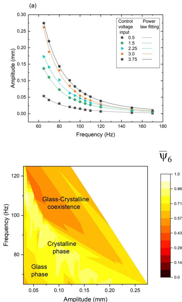
Fig. 5 (a) The amplitude  $A$  as a function of frequency  $f$  for different control voltages. The power laws fitting have an exponent of  $3.24 \pm 0.12$ . (b) Comparison of final particle configurations obtained in the glass-glass case for different frequencies and amplitudes at a constant particle number of 250. The coloured map shows the different phase regions formed by the different combinations of frequency and amplitude.
