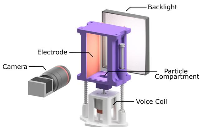
Fig. 1 Basic setup of the experiment (from ref. 27).
